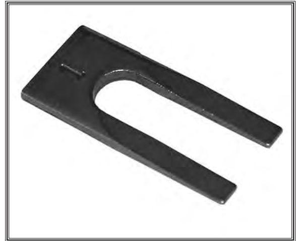
Figure 22. Chuck removal wedge.
