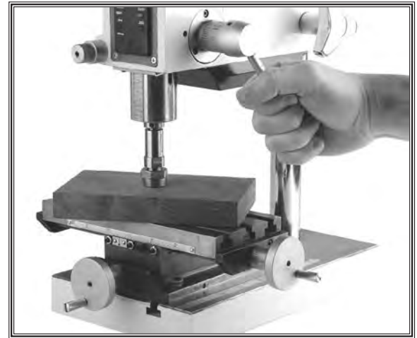
Figure 24. Installing the collet chuck.
