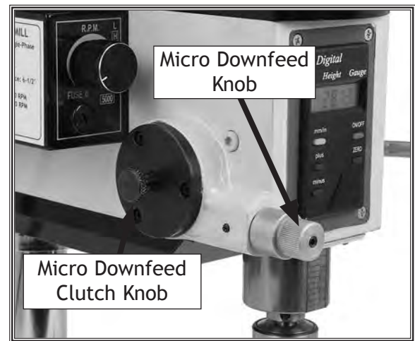
Figure 16. Micro downfeed controls.
