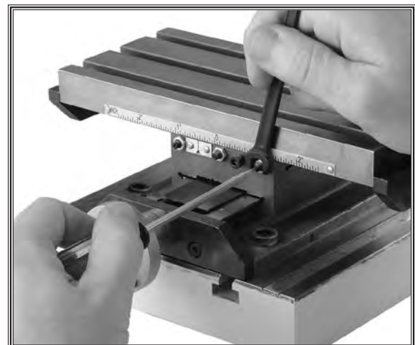
Figure 31. Longitudinal gib screw.
