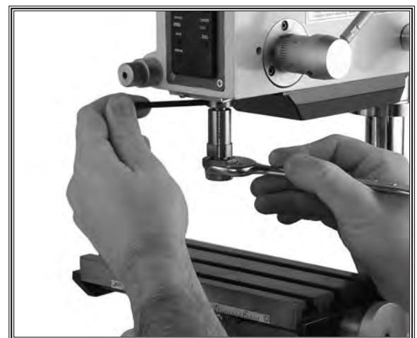
Figure 26. Installing a collet.
