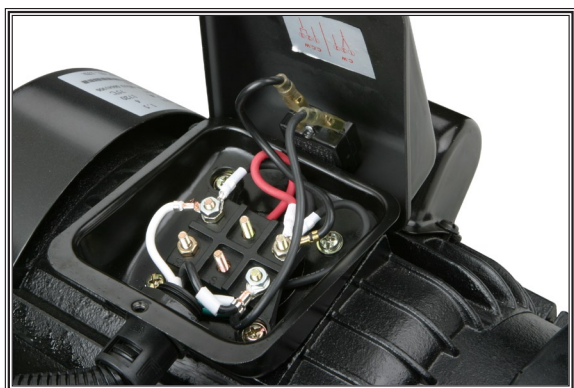
Figure 42. Junction box (M1).
