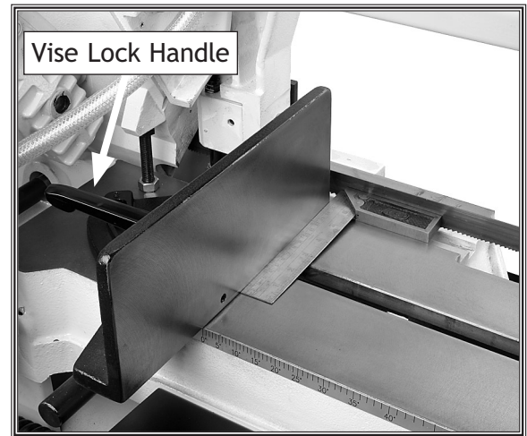
Figure 15. Squaring vise to blade.
