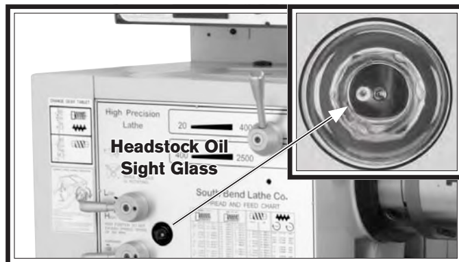
Figure 109. Location of the headstock oil sight glass.
