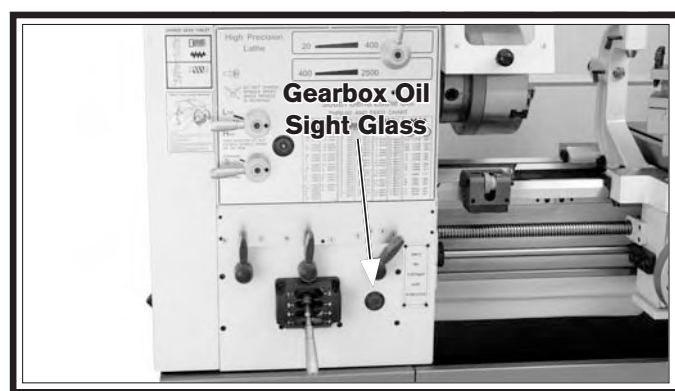
Figure 112. Gearbox sight glass location.
