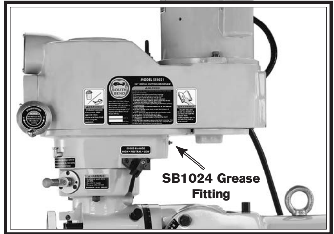
Figure 52. SB1024 headstock gearing grease fitting.
