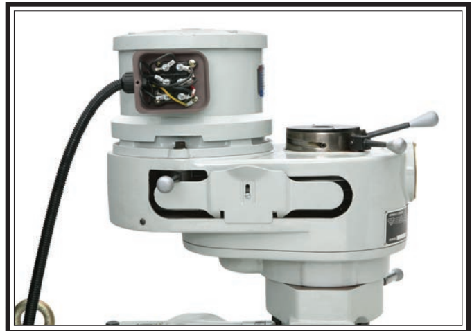
Figure 74. SB1025 Motor junction box.
