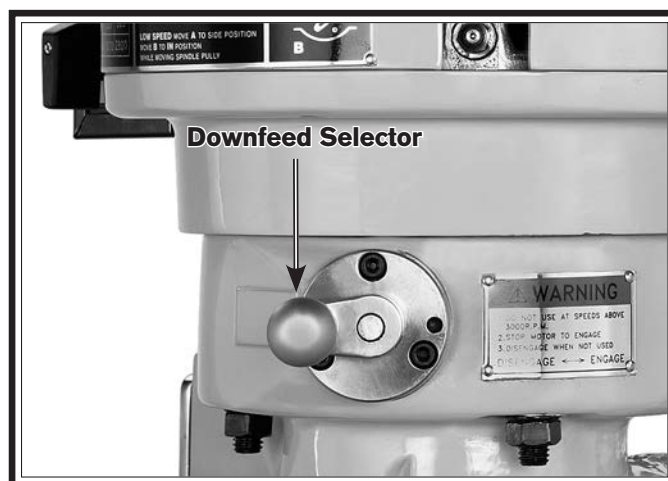
Figure 38. Downfeed selector in the manual (disengaged) position.
