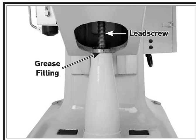
Figure 56. Table elevation leadscrew and grease fitting.
