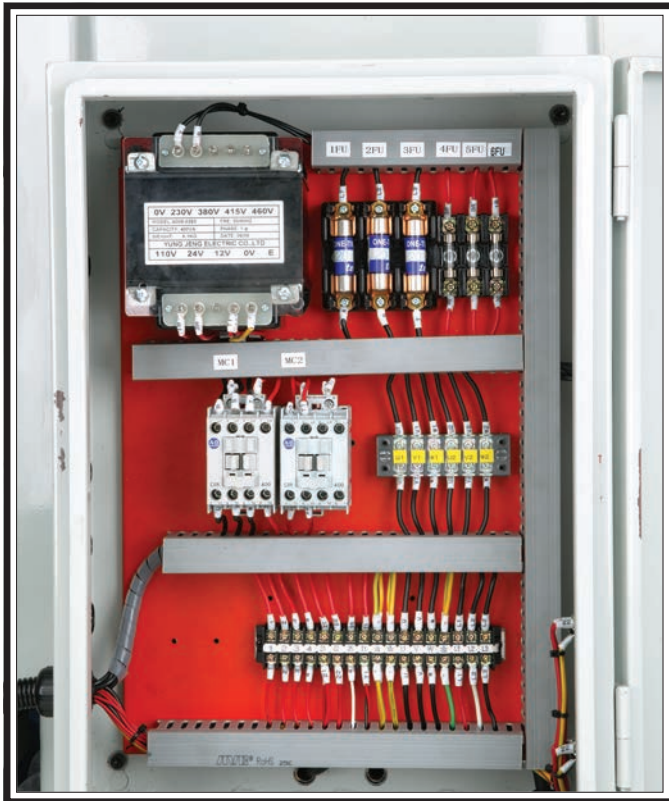
Figure 72. SB1025 Electrical box.
