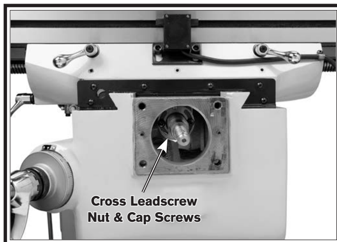
Figure 67. Cross leadscrew nut and cap screws.
