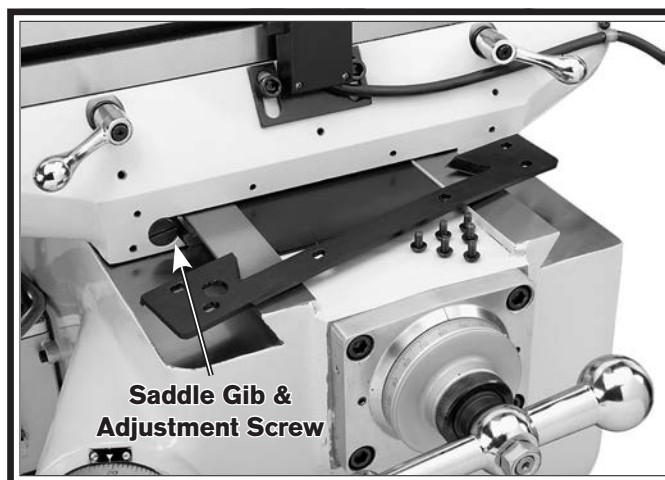
Figure 62. Saddle gib and adjustment screw.
