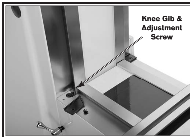
Figure 63. Knee gib and adjustment screw.
