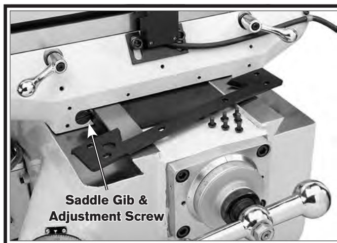
Figure 62. Saddle gib and adjustment screw.
