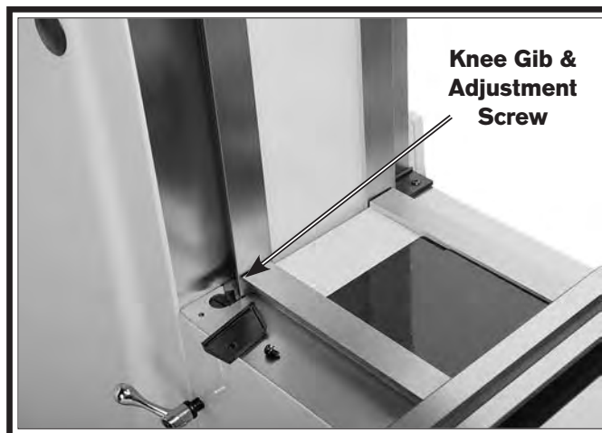
Figure 63. Knee gib and adjustment screw.
