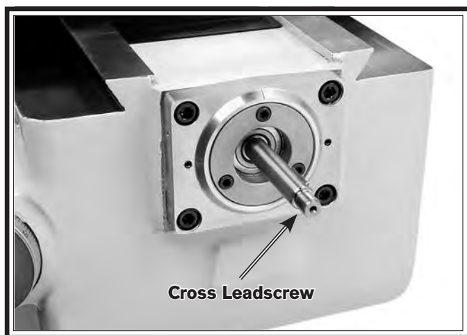
Figure 65. Ball handle, rings, and key removed from the cross leadscrew.
