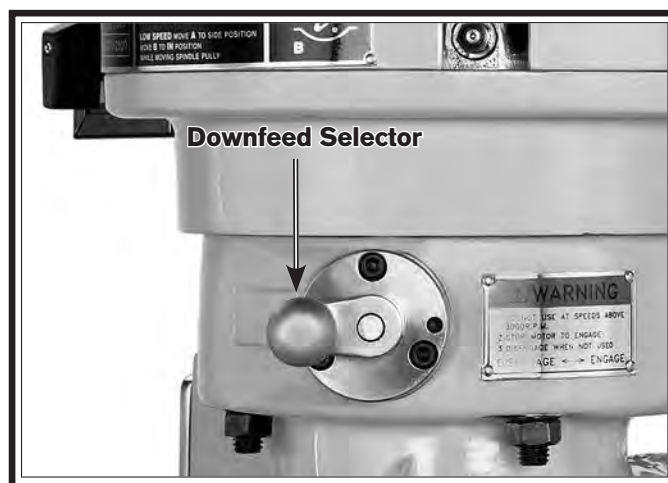
Figure 38. Downfeed selector in the manual (disengaged) position.
