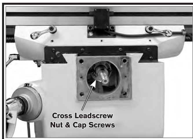
Figure 67. Cross leadscrew nut and cap screws.
