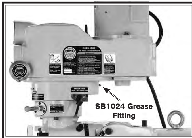
Figure 52. SB1024 headstock gearing grease fitting.
