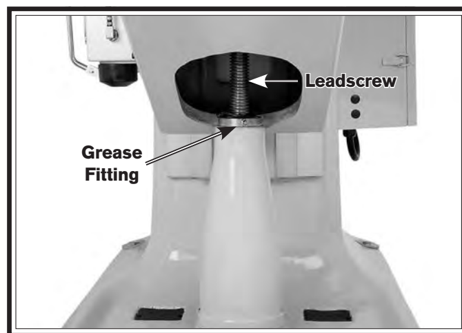
Figure 56. Table elevation leadscrew and grease fitting.
