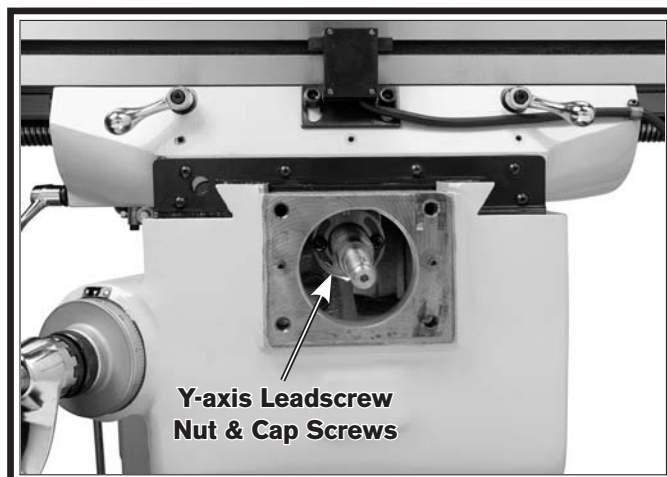
Figure 66. Y-axis leadscrew nut and cap screws.
