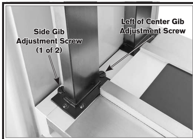
Figure 62. Knee gib adjustment screws.
