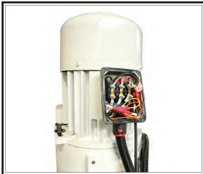
Figure 70. Spindle motor wiring.
