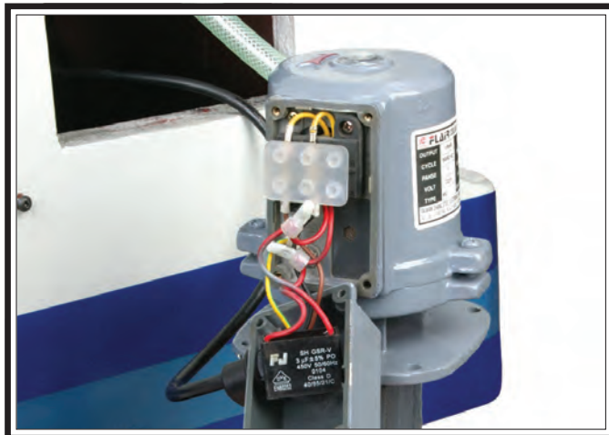
Figure 72. Coolant pump motor wiring.
