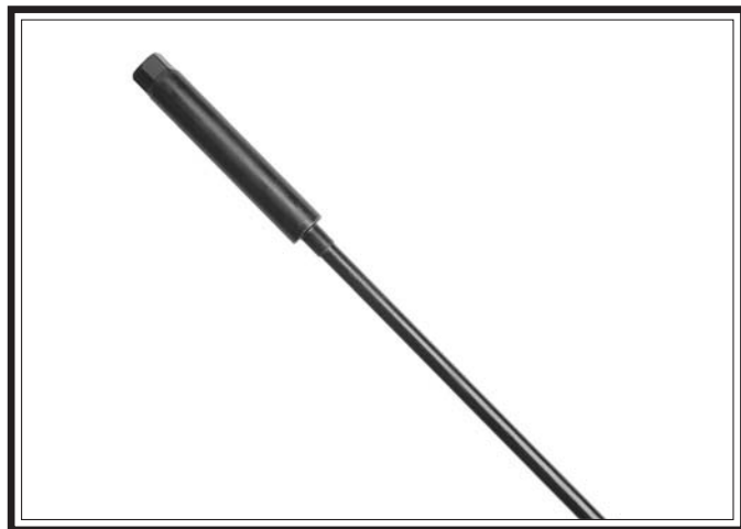
Figure 46. Spindle drawbar and spacer.
