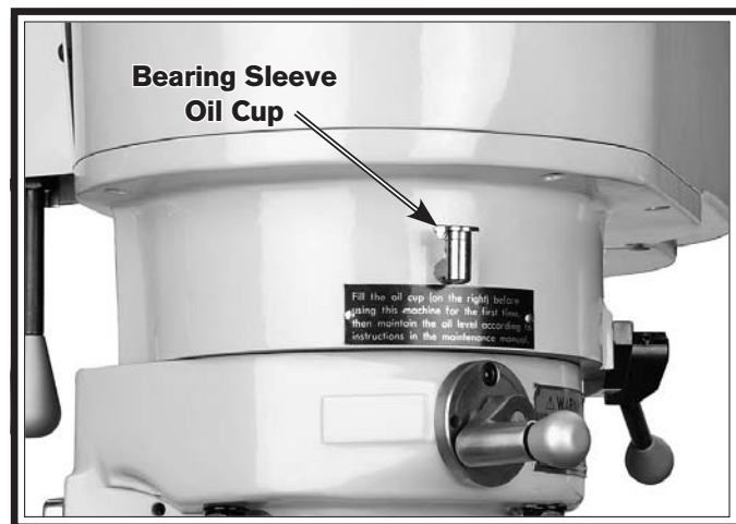
Figure 51. Speed range bearing sleeve.
