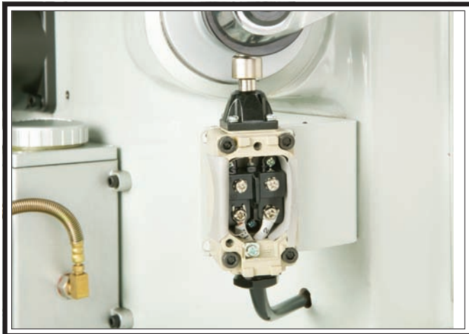
Figure 74. Z-axis crank safety switch.
