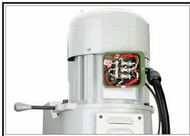
Figure 70. Spindle motor wiring.
