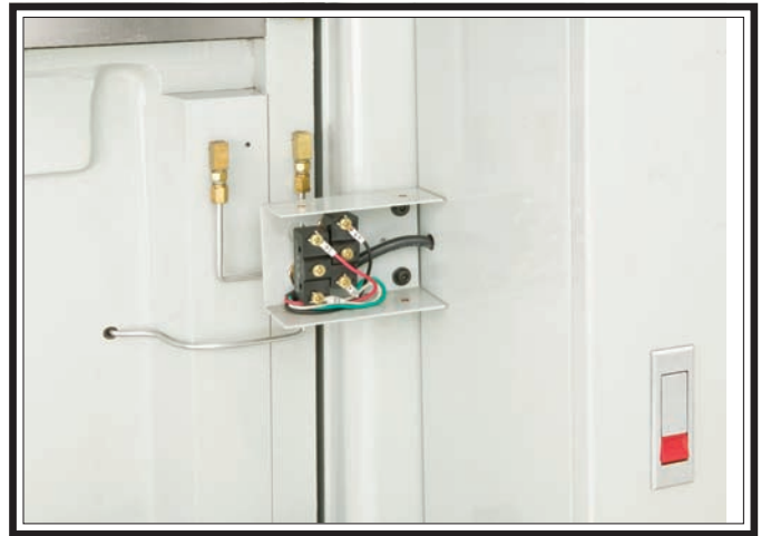
Figure 75. Z-axis limit switches.
