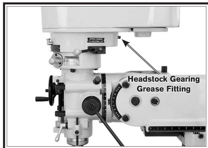
Figure 52. Headstock gearing grease fitting.
