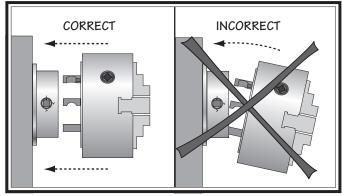
Figure 31. Inserting camlock studs into spindle cam
