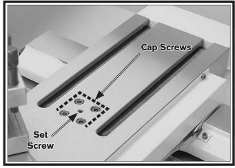
Figure 112. Cross slide backlash adjustment screws.
