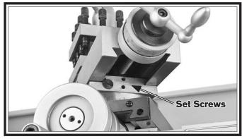
Figure 111. Compound rest backlash adjustment set screws.
