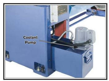
Figure 141. Coolant pump location.
