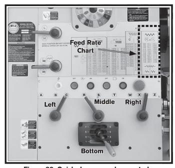
Figure 69. Quick-change gearbox controls.
