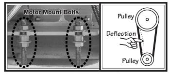
Figure 121. V-belt adjustment.
