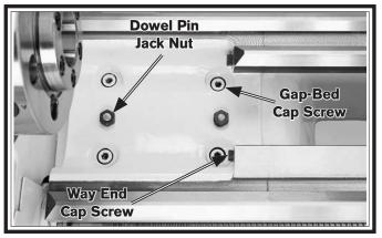
Figure 136. Fasteners holding gap in place.
