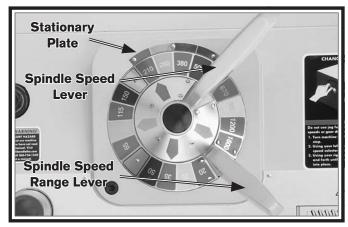
Figure 26. Spindle speed set at 210 RPM.
