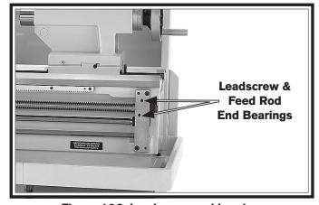
Figure 106. Leadscrew end bearing.
