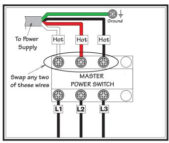
Figure 137. Swapping L1 and L2 power connections to correct out-of-phase wiring.
