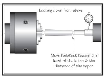
Figure 49. Adjust tailstock away from the operator.
