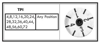
Figure 82. Any position on the dial for threading TPI divisible by 4.
