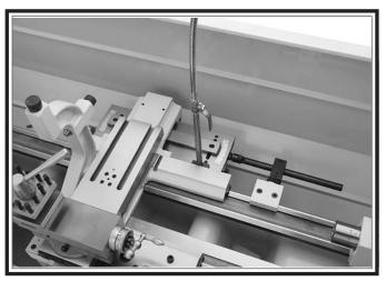
Figure 95. Model SB1271 Taper Attachment.
