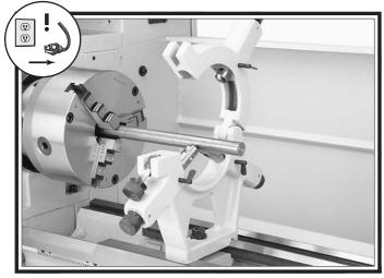
Figure 56. Workpiece mounted in the steady rest.
