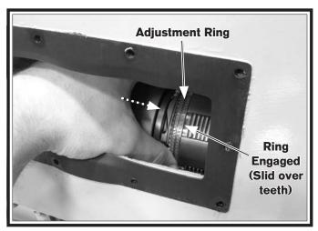
Figure 126. Engaging adjustment ring (reverse side shown).
