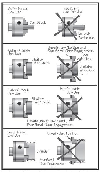
Figure 36. Jaw selection and workpiece holding.
