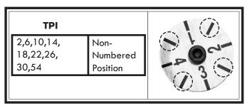
Figure 83. Marks are selected on the dial for threading even TPI not divisible by 4.
