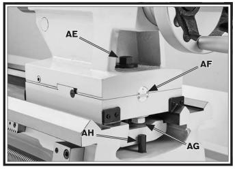
Figure 8. Tailstock controls.
