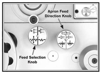
Figure 70. Apron feed selection and direction knobs.
