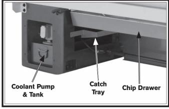
Figure 109. Additional coolant components.
