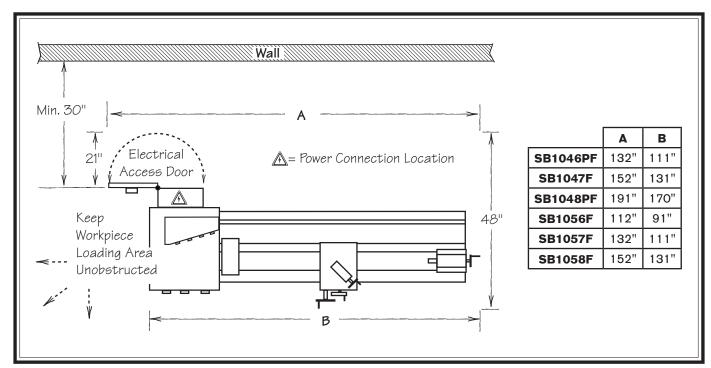
Figure 13. Space required for full range of movement.
