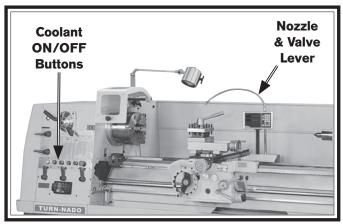
Figure 108. Coolant controls.
