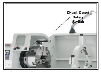
Figure 144. Chuck Guard Safety switch location.
