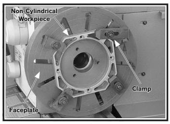
Figure 39. Example photo of workpiece clamped in a faceplate.
