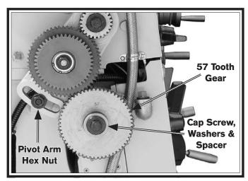
Figure 76. End gear components.
