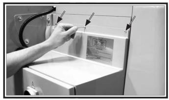
Figure 122. Removing electrical cabinet fasteners.
