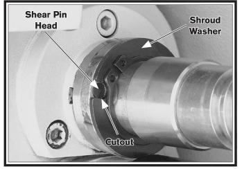
Figure 129. Shroud washer and shear pin alignment.
