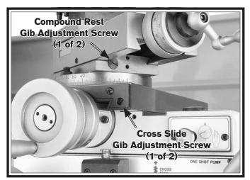
Figure 114. Compound and cross slide gib adjustment screws.
