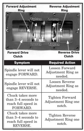
Figure 124. Clutch adjustment overview.
