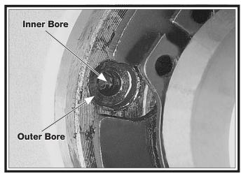
Figure 131. Shear pin bores aligned.
