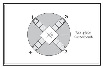
Figure 37. 4-jaw tightening sequence.
