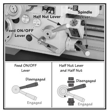
Figure 28. Apron controls for test run.
