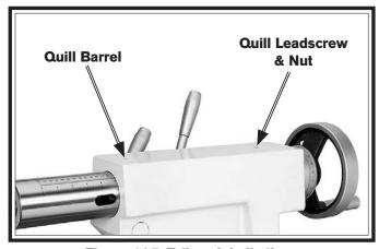
Figure 105. Tailstock ball oilers.
