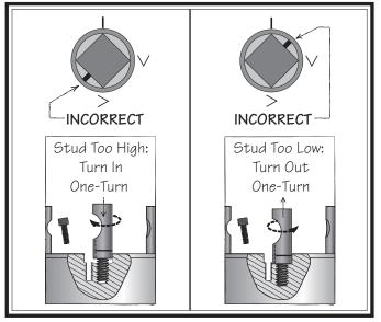
Figure 33. Correcting an improperly installed stud.
