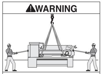
This machine and its parts are heavy! Serious personal injury may occur if safe moving methods are not used. To reduce the risk of a lifting or dropping injury, ask others for help, and use power equipment and guide rods.
