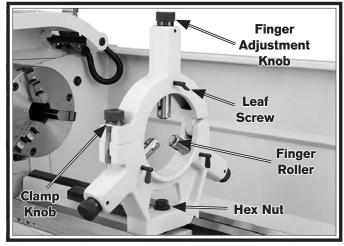
Figure 55. Steady rest components.
