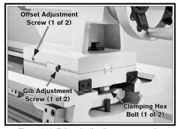
Figure 118. Tailstock gib adjustment controls.
