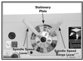
Figure 66. Spindle speed of 1600 RPM is selected.
