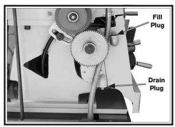
Figure 100. Locations of the quick-change gearbox fill and drain plugs.
