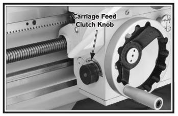
Figure 71. Adjustable carriage feed clutch knob.
