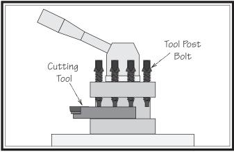
Figure 60. Example of tool mounted in tool post.
