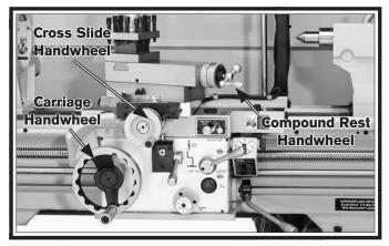
Figure 64. Carriage controls for manual feed.
