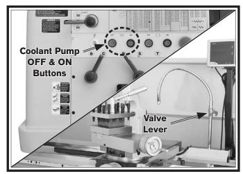
Figure 89. Coolant flow controls.
