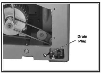
Figure 98. Headstock oil drain plug.
