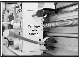
Figure 117. Carriage lock clamp.
