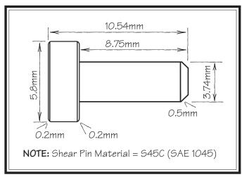
Figure 127. Shear pin specifications.
