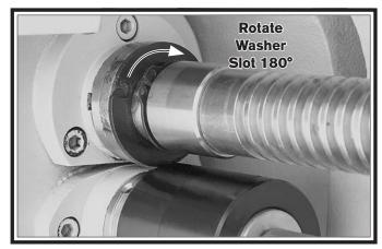
Figure 133. Shroud washer positioning.
