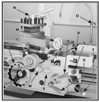
Figure 5. Carriage controls.
