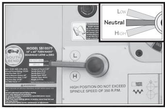
Figure 67. Gearbox range lever.
