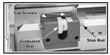
Figure 63. Micrometer stop.
