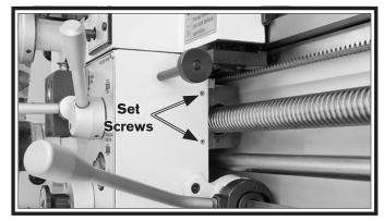
Figure 119. Half nut gib adjustment.
