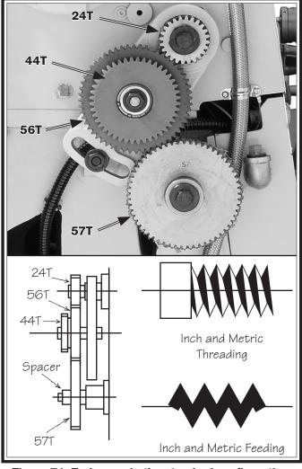
Figure 74. End gears in the standard configuration.
