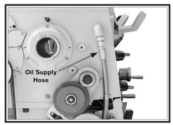
Figure 97. Headstock oil supply hose.
