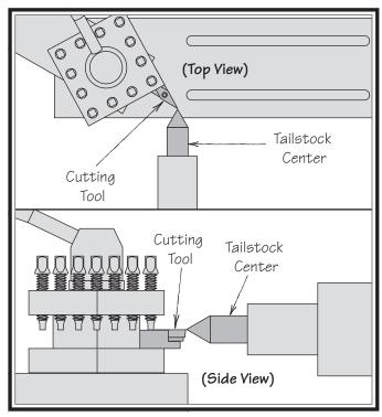
Figure 62. Cutting tool tip aligned with tailstock center.
