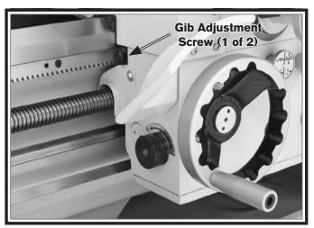
Figure 116. Front saddle gib adjustment screw.
