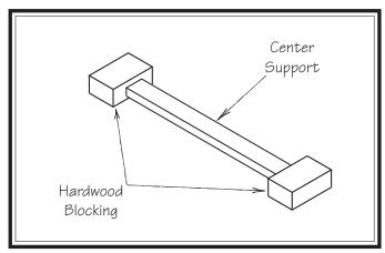
Figure 15. Example of blocking center support.
