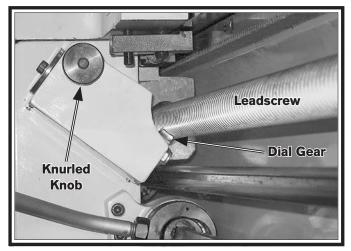
Figure 80. Thread dial engaged with the leadscrew.
