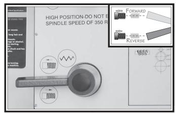
Figure 68. Headstock feed direction lever.
