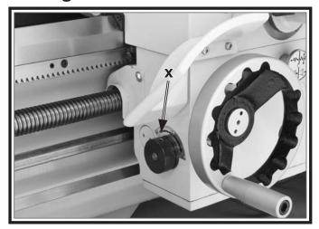
Figure 6. Adjustable carriage feed clutch knob.
