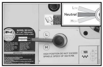
Figure 27. Gearbox range lever in neutral.
