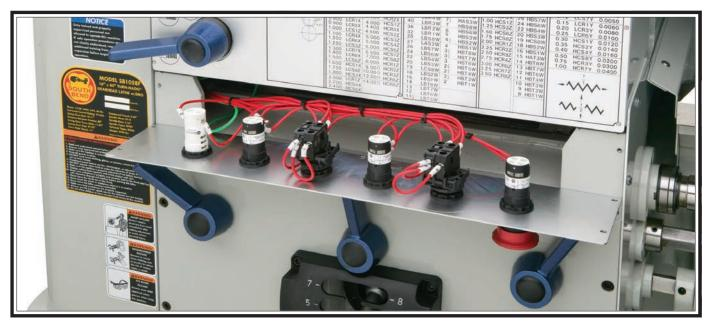
Figure 142. Control panel wiring.
