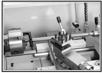
Figure 47. Example photo of stock mounted between the centers.
