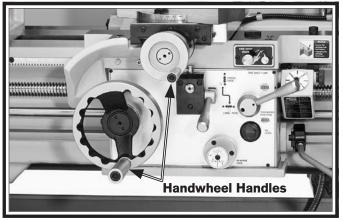
Figure 20. Handwheel handles installed.
