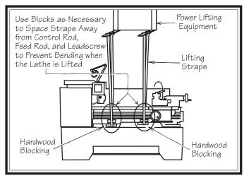
Figure 16. Example of lathe setup for lifting.
