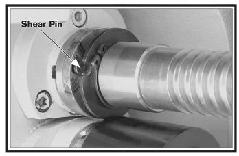
Figure 132. New shear pin installed in bore.
