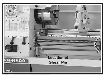
Figure 128. Location of shear pin.
