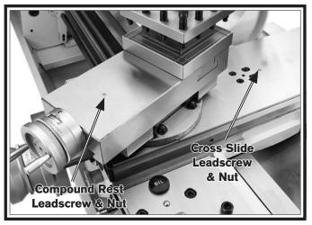
Figure 104. Carriage ball oilers.
