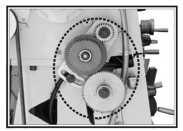
Figure 107. End gears.
