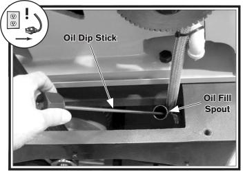
Figure 96. Checking headstock oil tank level.
