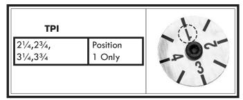
Figure 86. Position for 1/4 or 3/4 fractional TPI.
