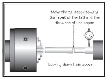
Figure 48. Adjust tailstock toward the operator.
