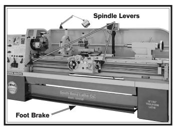
Figure 9. Foot brake and spindle levers.
