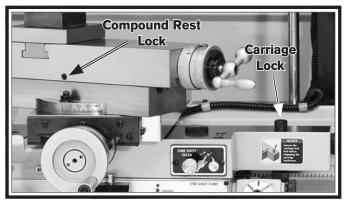
Figure 58. Compound rest and carriage locks.
