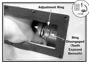
Figure 125. Disengaging adjustment ring (reverse side shown).
