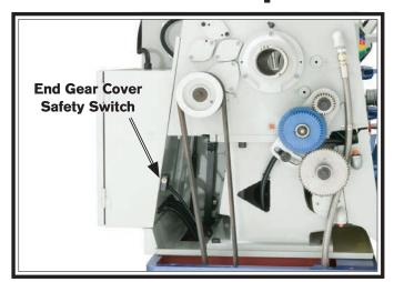
Figure 143. End Gear Cover Safety switch location.
