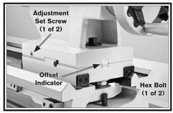
Figure 44. Tailstock offset controls.
