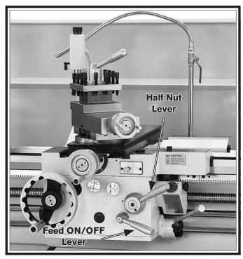
Figure 78. Carriage controls.
