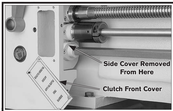
Figure 139. Location of clutch front cover (side cover removed for photo clarity).
