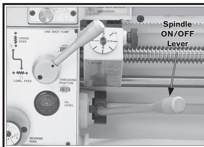
Figure 33. Spindle ON/OFF lever in the OFF (middle) position.
