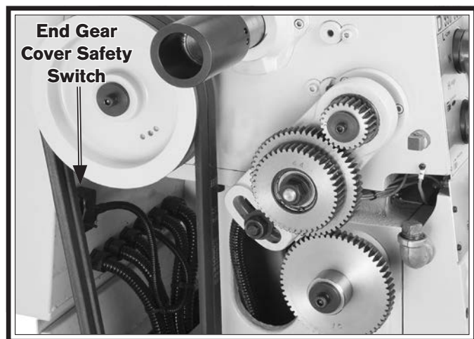
Figure 156. End Gear Cover Safety Switch location.
