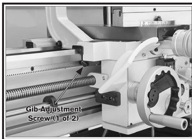
Figure 126. Front saddle gib adjustment screw.
