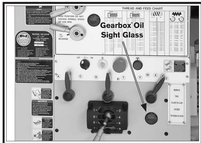
Figure 108. Location of quick-change gearbox oil sight glass.
