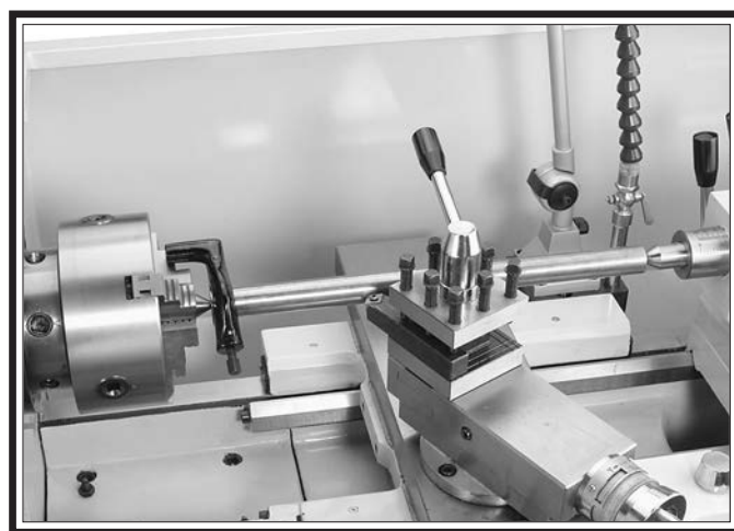
Figure 60. Example photo of a workpiece mounted between the centers.
