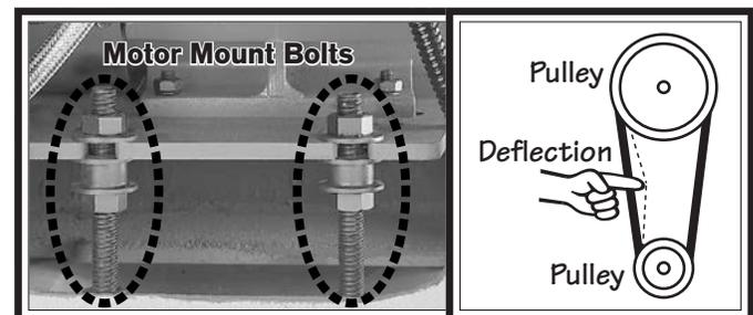
**Figure 121. V-belt adjustment.**
