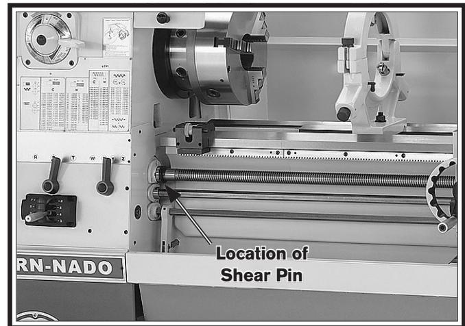
**Figure 128. Location of shear pin.**
