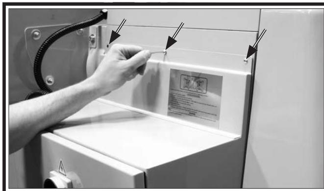
**Figure 122. Removing electrical cabinet fasteners.**
