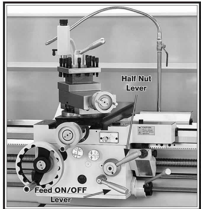
Figure 78. Carriage controls.
