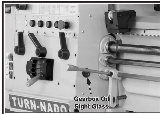
**Figure 99. Location of quick-change gearbox oil sight glass.**
