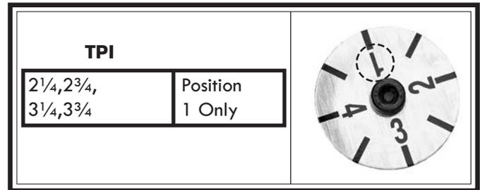
**Figure 86.** Position for ¼ or ¾ fractional TPI.
