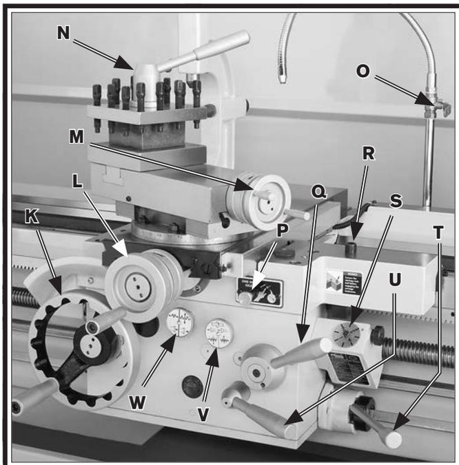
Figure 5. Carriage controls.
