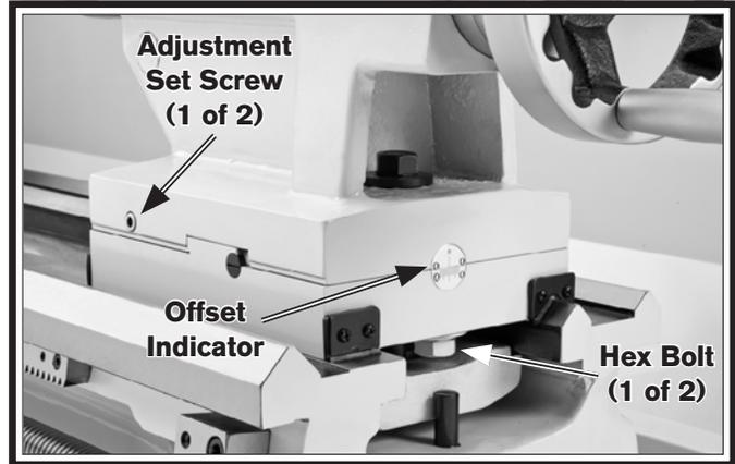
**Figure 44.** Tailstock offset controls.
