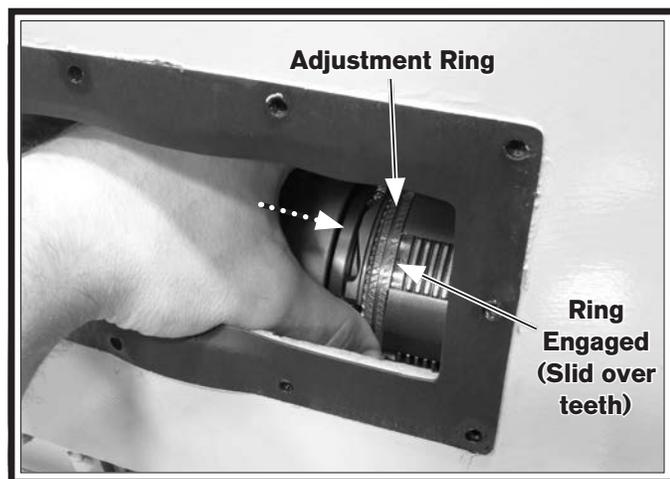
**Figure 126.** Engaging adjustment ring (reverse side shown).
