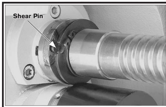
**Figure 132. New shear pin installed in bore.**
