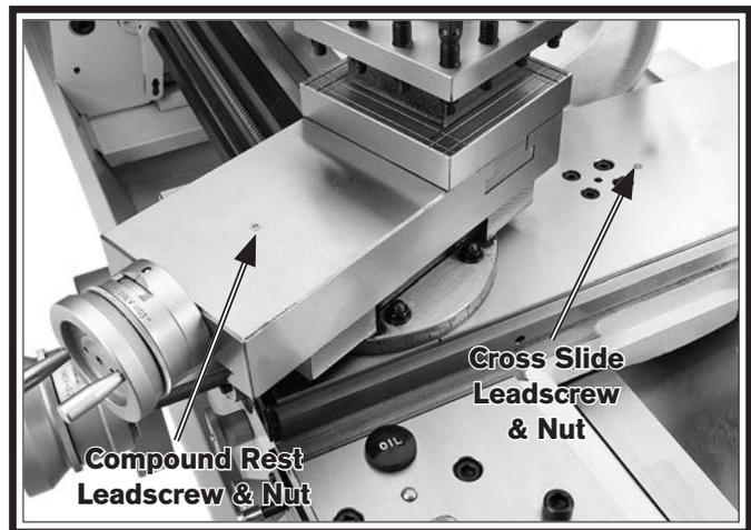
Figure 104. Carriage ball oilers.
