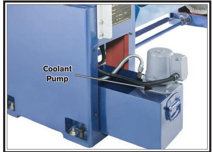
Figure 141. Coolant pump location.
