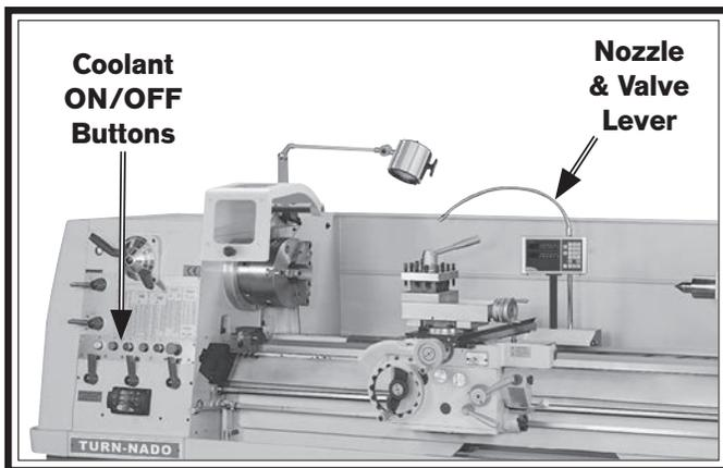
Figure 108. Coolant controls.
