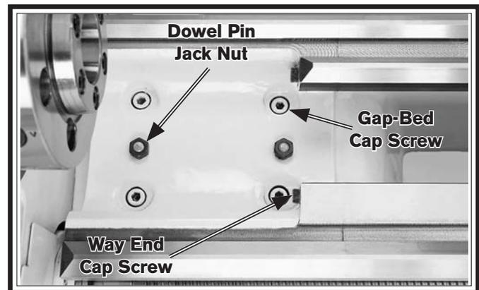
**Figure 136.** Fasteners holding gap in place.
