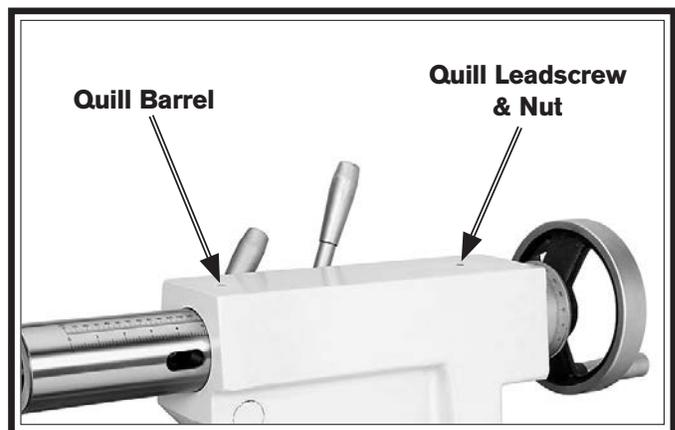
Figure 105. Tailstock ball oilers.
