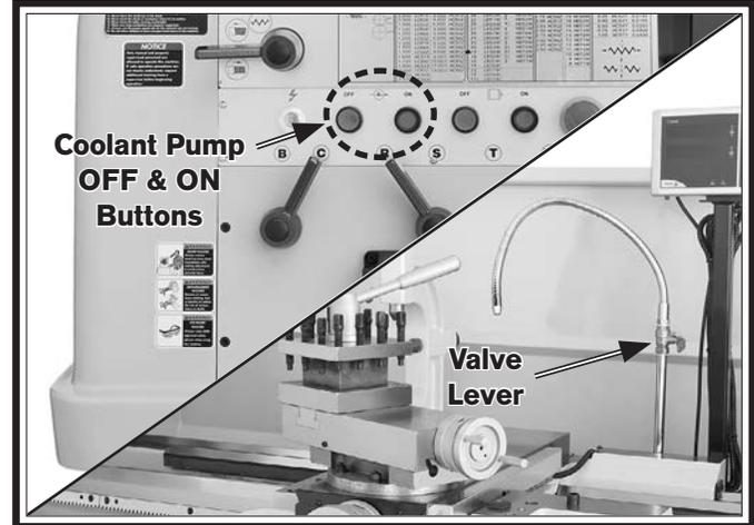
**Figure 89. Coolant flow controls.**
