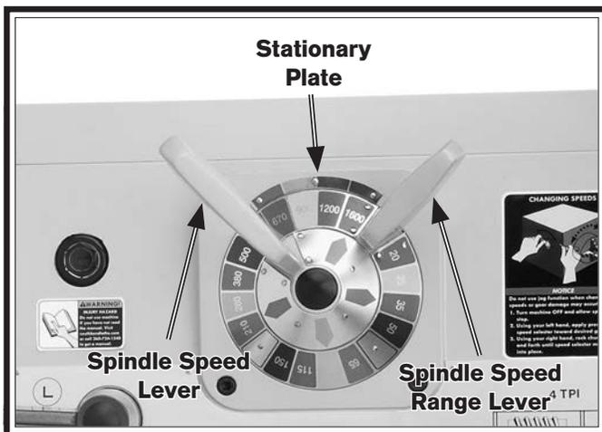
**Figure 66. Spindle speed of 1600 RPM is selected.**
