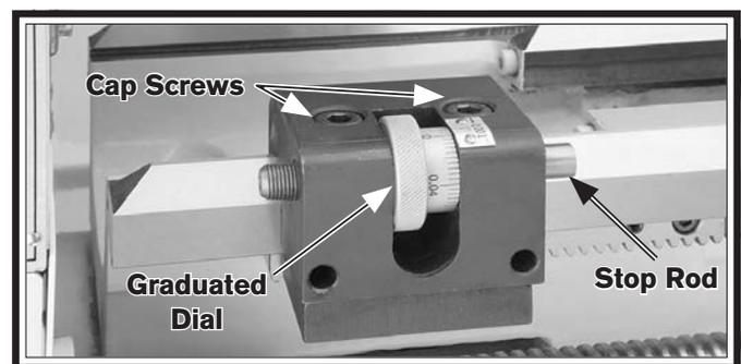
**Figure 63. Micrometer stop.**
