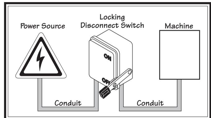
**Figure 21.** Typical hardwire setup with a locking disconnect switch.
