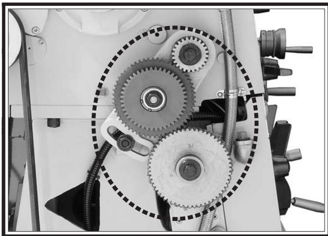
**Figure 107. End gears.**
