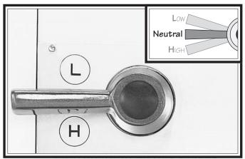
Figure 27. Gearbox range lever in neutral.
