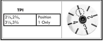
Figure 87. Position for  $\frac{1}{4}$  or  $\frac{3}{4}$  fractional TPI.
