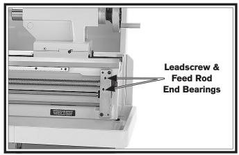
Figure 110. Leadscrew end bearing.
