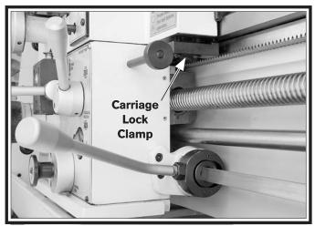
Figure 121. Carriage lock clamp.
