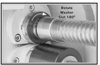
Figure 137. Shroud washer positioning.
