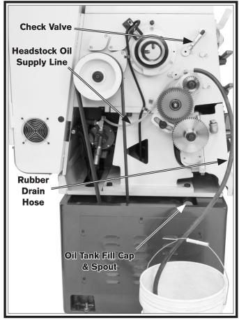
Figure 101. Draining headstock oil.
