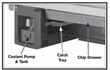
Figure 113. Additional coolant components.
