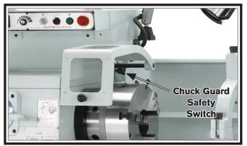
Figure 151. Chuck guard limit switch.
