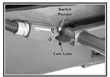
Figure 129. Brake switch.
