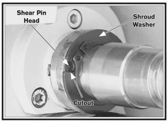
Figure 133. Shroud washer and shear pin alignment.
