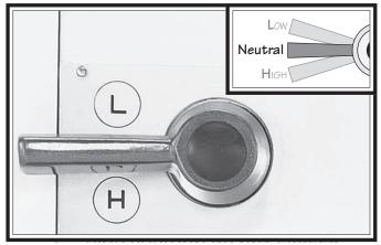
Figure 68. Gearbox range lever.
