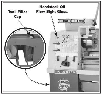
Figure 99. Headstock oil flow sight glass location.
