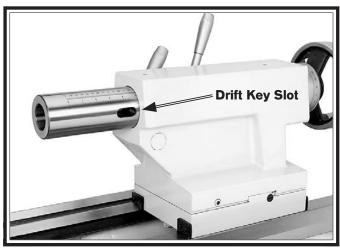
Figure 53. Drift key slot in the side of the quill.
