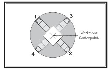
Figure 37. 4-jaw tightening sequence.
