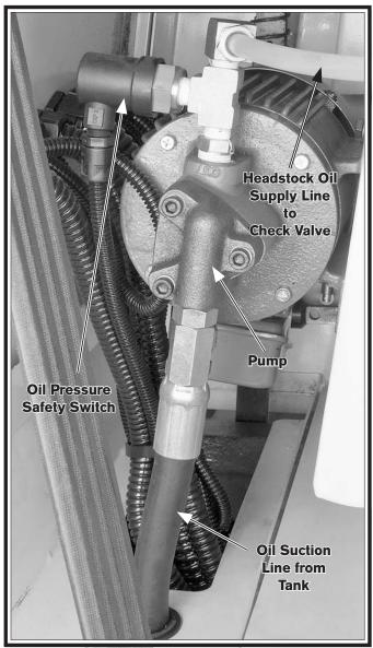
Figure 98. Oil pump and oil pressure safety switch.
