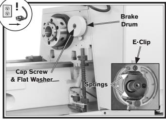
Figure 130. Brake drum.
