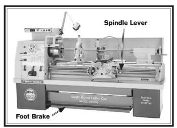
Figure 9. Foot brake and spindle lever.
