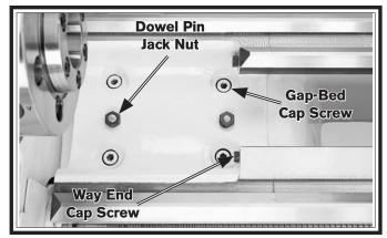
Figure 140. Fasteners holding gap in place.
