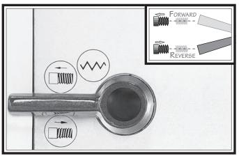
Figure 69. Headstock feed direction lever.
