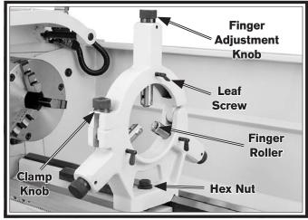
Figure 55. Steady rest components.
