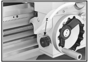
Figure 6. Adjustable carriage feed clutch knob.
