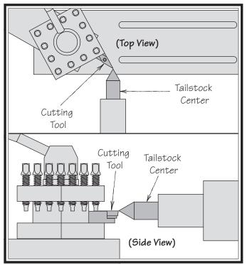
Figure 62. Cutting tool tip aligned with tailstock center.
