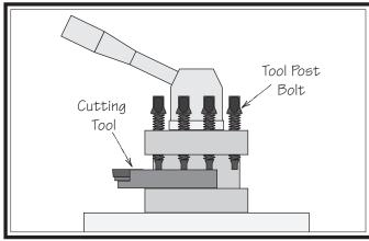
Figure 60. Example of tool mounted in tool post.
