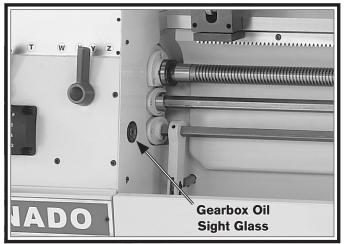
Figure 103. Location of quick-change gearbox oil sight glass.
