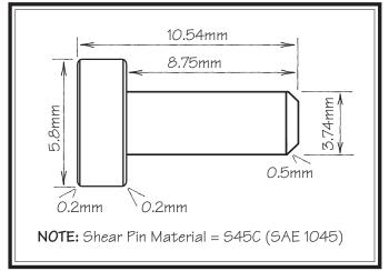
Figure 131. Shear pin specifications.
