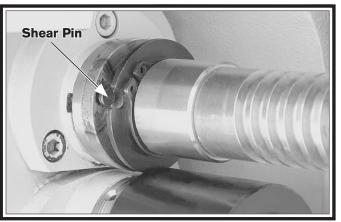
Figure 136. New shear pin installed in bore.
