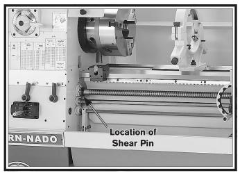
Figure 132. Location of shear pin.
