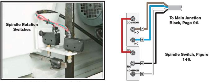
Figure 146. Spindle rotation switch location.
