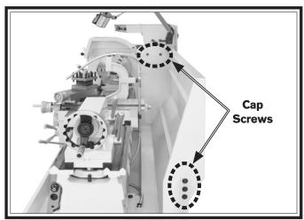
Figure 126. Locations of the backsplash cap screws.
