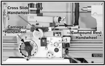
Figure 64. Carriage controls for manual feed.
