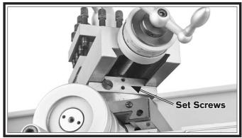
Figure 115. Compound rest backlash adjustment set screws.
