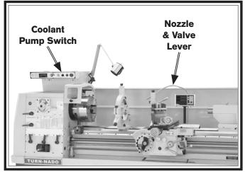
Figure 90. Coolant system controls.
