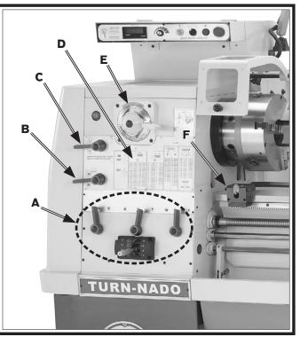
Figure 3. Headstock controls.
