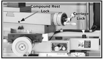
Figure 58. Compound rest and carriage locks.
