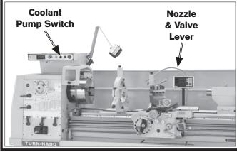
Figure 112. Coolant controls.
