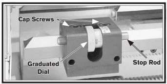
Figure 63. Micrometer stop.
