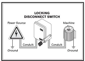
Figure 10. Typical hardwire setup with a locking disconnect switch.
