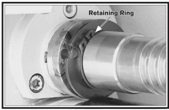
Figure 134. Shear pin access.
