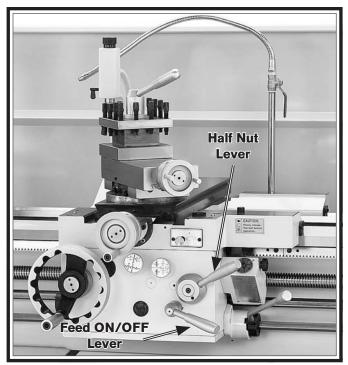
Figure 79. Carriage controls.
