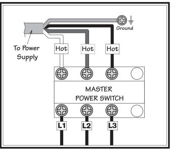
Figure 23. Power connection at master power switch.
