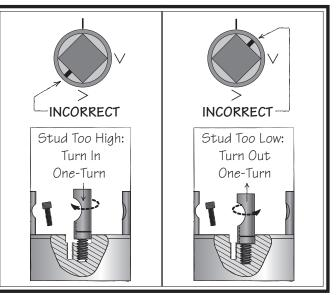
Figure 33. Correcting an improperly installed stud.
