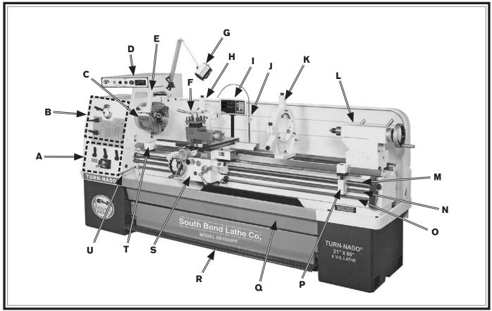
Figure 1. General identification (Model SB1043PF shown).
