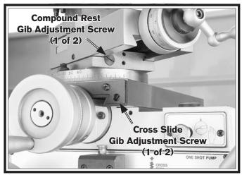
Figure 118. Compound and cross slide gib adjustment screws.
