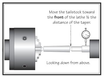
Figure 48. Adjust tailstock toward the operator.
