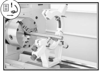
Figure 56. Workpiece mounted in the steady rest.
