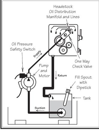
Figure 97. Lubrication system overview.
