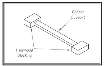
Figure 15. Example of blocking center support.
