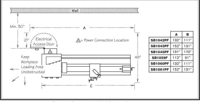
Figure 13. Space required for full range of movement.
