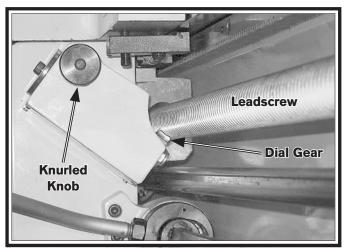
Figure 81. Thread dial engaged with the leadscrew.
