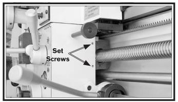
Figure 123. Half nut gib adjustment.
