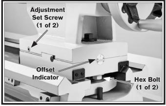
Figure 44. Tailstock offset controls.
