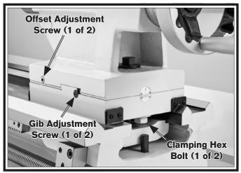
Figure 122. Tailstock gib adjustment controls.
