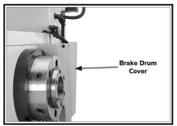
Figure 128. Brake drum cover.
