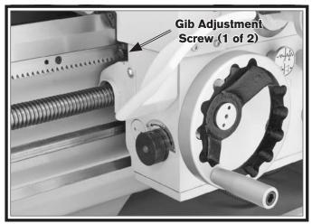
Figure 120. Front saddle gib adjustment screw.
