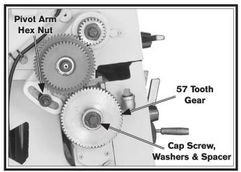
Figure 77. End gear components.
