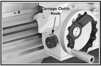
Figure 72. Adjustable carriage feed clutch knob.
