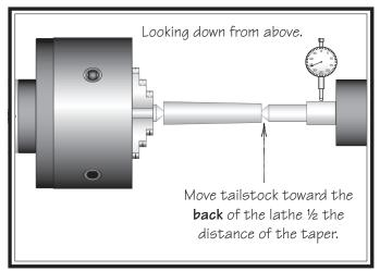
Figure 49. Adjust tailstock away from the operator.
