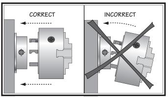
Figure 31. Inserting camlock studs into spindle cam holes.
