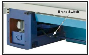
Figure 150. Brake switch location.
