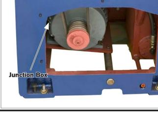
Figure 144. Spindle motor location.
