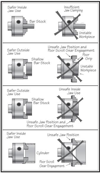
Figure 36. Jaw selection and workpiece holding.
