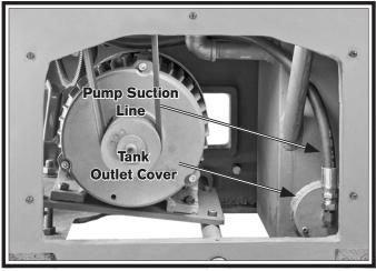
Figure 102. Location of tank outlet cover.
