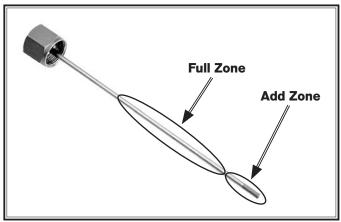
Figure 100. Headstock oil level dip stick.
