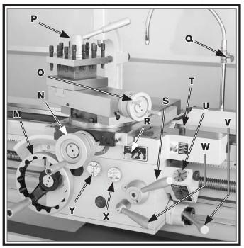
Figure 5. Carriage controls.
