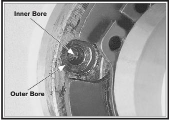
Figure 135. Shear pin bores aligned.
