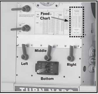
Figure 70. Quick-change gearbox controls.
