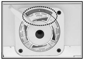
Figure 26. Spindle speed range lever.
