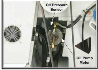
Figure 145. Oil pump motor & pressure sensor location.
