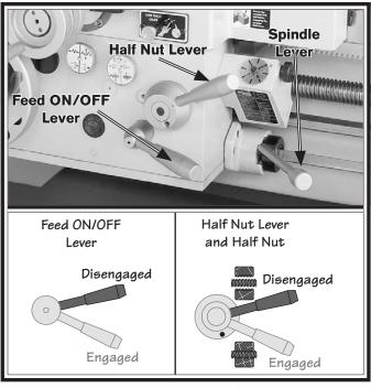
Figure 28. Apron controls for test run.
