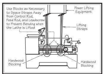
Figure 16. Example of lathe setup for lifting.
