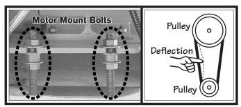
Figure 125. V-belt adjustment.
