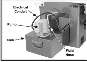
Figure 114. Coolant tank and pump.
