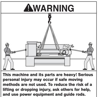
Do not attempt to lift or move this lathe without using the proper lifting equipment (such as forklift or crane) or the necessary assistance from other people. Each piece of lifting equipment must be rated for at least 25% more than the shipping weight of your lathe to support dynamic loads that may be applied while lifting. Refer to **Things You'll Need** on **Page 21** for details.
