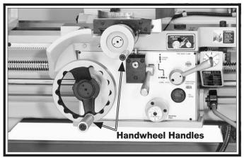
Figure 20. Handwheel handles installed.
