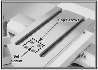
Figure 116. Cross slide backlash adjustment screws.
