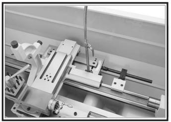
Figure 96. Model SB1271 Taper Attachment.
