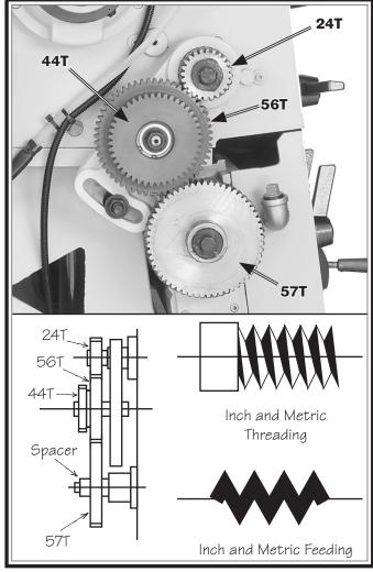
Figure 75. End gears in the standard configuration.
