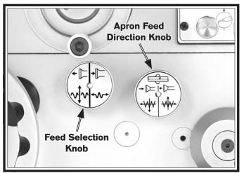
Figure 71. Apron feed selection and direction knobs.
