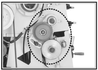
Figure 111. End gears.
