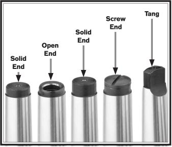
Figure 41. Types of tapered arbors and tooling.
