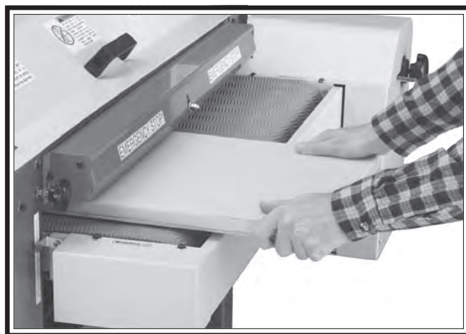
Figure 26. Example of using D3003 PRO-STIK® cleaning pad to clean sandpaper.
