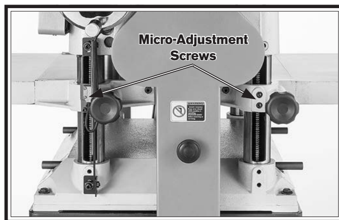
Figure 67. Location of table micro-adjustment screws (only one side shown).
