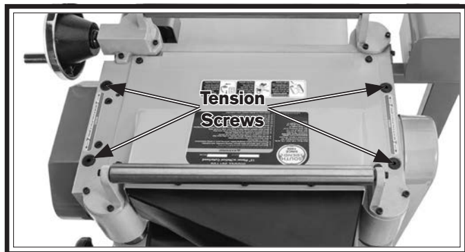
Figure 58. Feed-roller spring tension adjustment screws.
