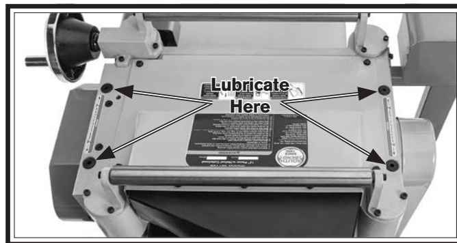
Figure 39. Lubrication locations for feed roller bushings.
