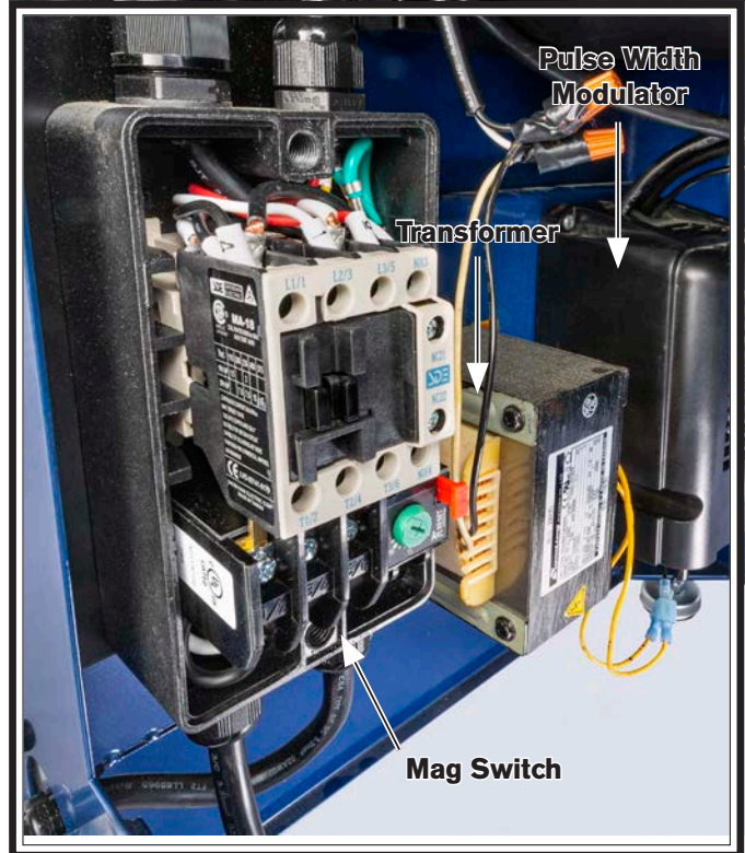
Figure 71. SB1108 mag switch, transformer, & pulse width modulator.
