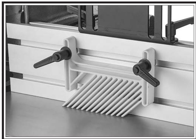
Figure 31. Example of featherboard installed on fence face.
