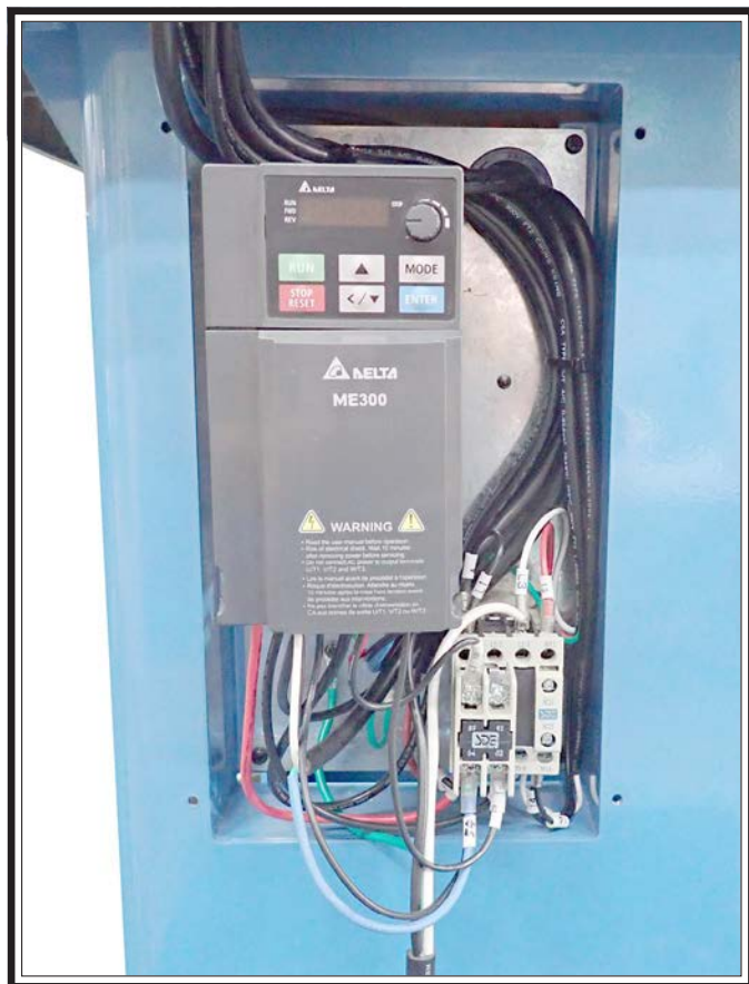
Figure 106. SB1119 electrical box wiring.
