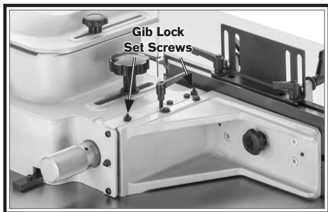
Figure 87. Location of fence gib lock set screws.
