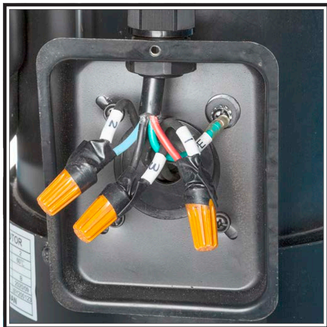
Figure 107. Motor junction box wiring.
