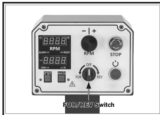
Figure 32. Location of FOR/REV switch.
