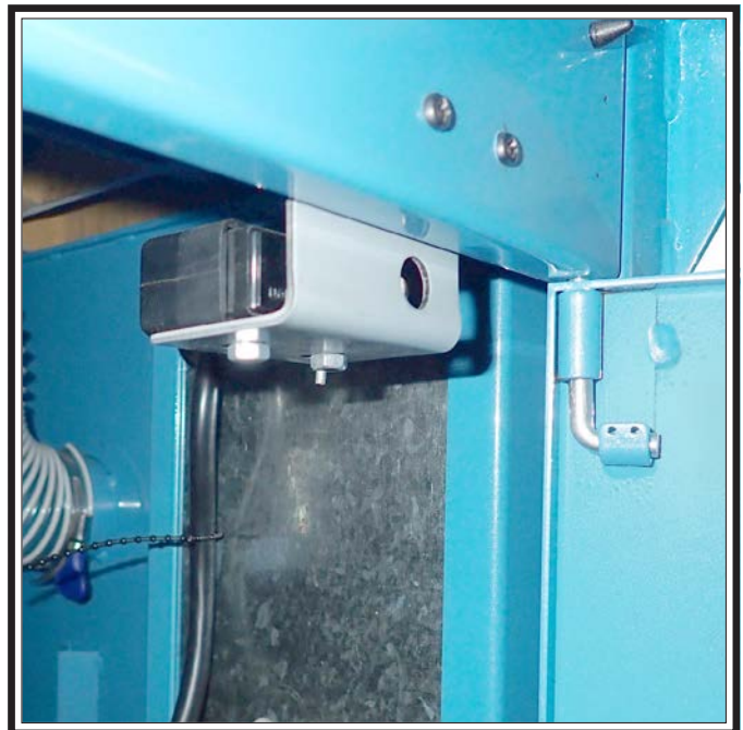
Figure 105. Cabinet door limit switch.
