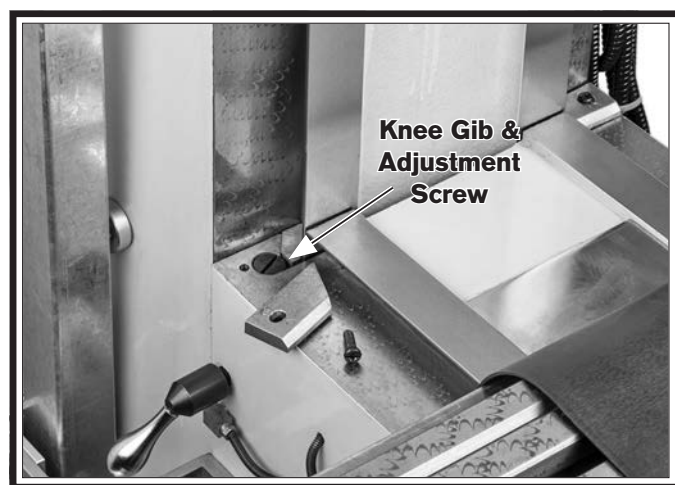
Figure 88. Knee gib and adjustment screw.
