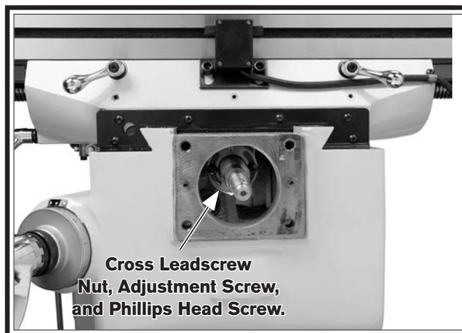
Figure 92. Example of cross leadscrew nut, adjustment screw, and Phillips head screw.
