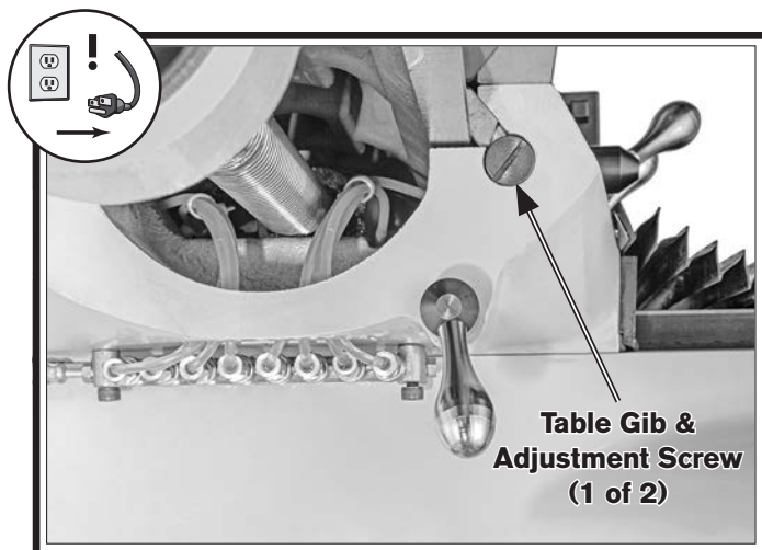
Figure 86. Table gib and adjustment screw underneath left side of table.
