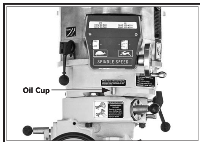
Figure 71. Oil cup location for speed range bearing sleeve.
