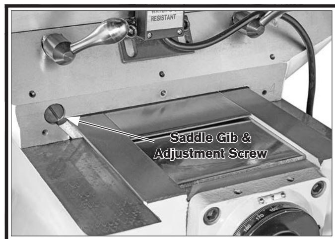
Figure 87. Saddle gib and adjustment screw.
