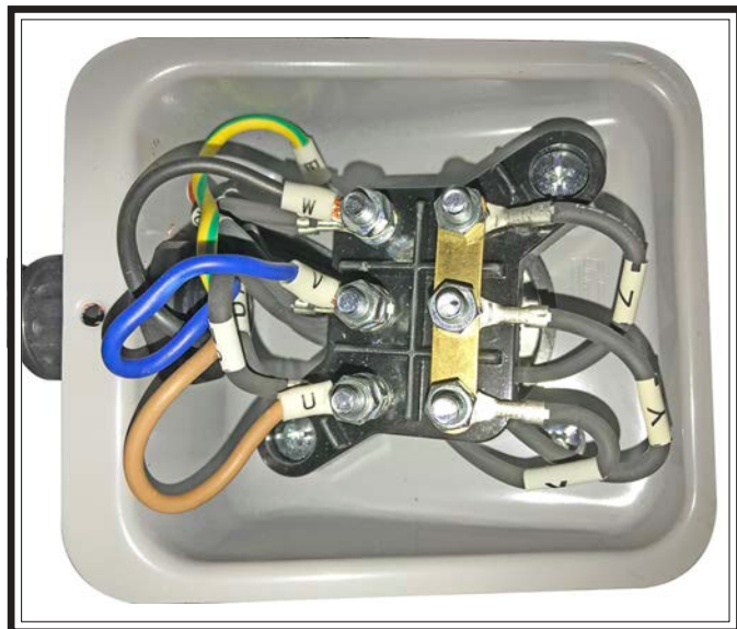
Figure 98. Motor wiring (220V).
