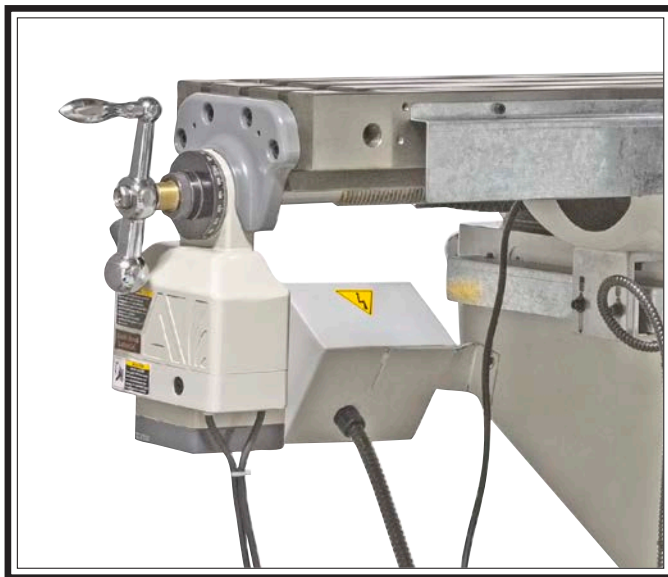
Figure 96. Power feed wiring.
