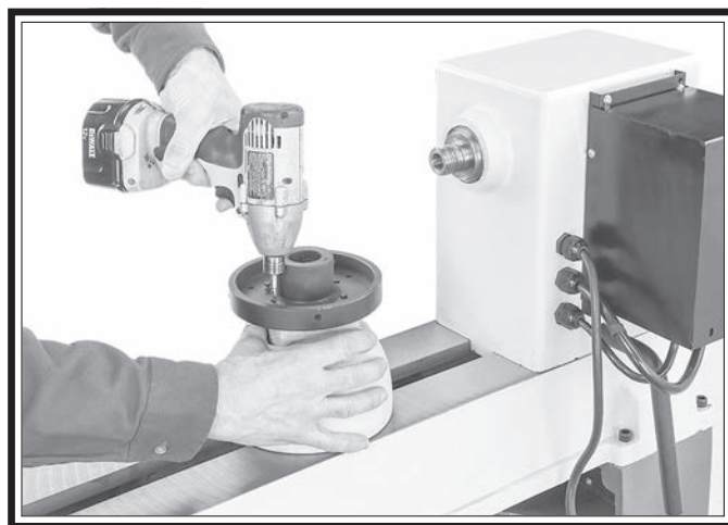
Figure 36. Typical attachment of faceplate to workpiece.
