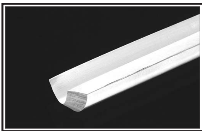
Figure 41. Example of a gouge.
