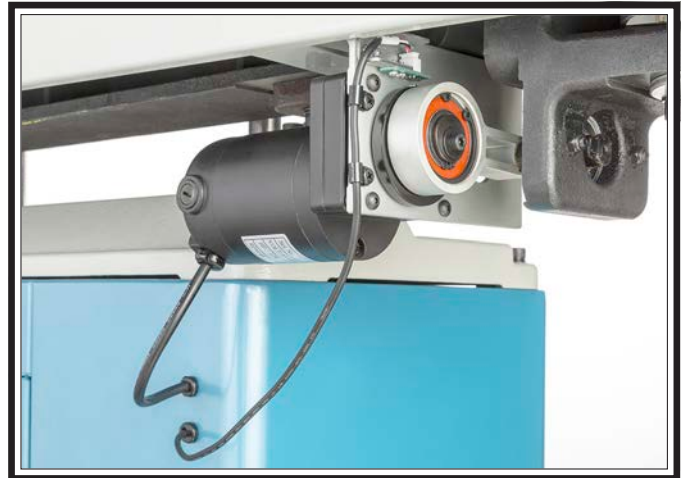
Figure 61. Oscillation motor and sensor.
