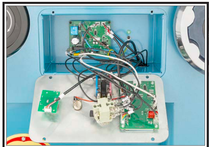
Figure 63. Control panel wiring.
