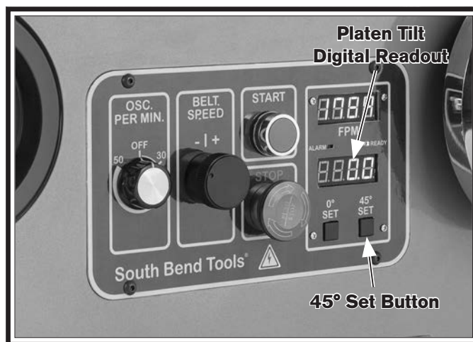
Figure 56. Location of platen tilt calibration components.
