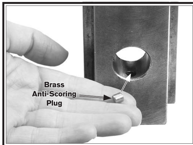
Figure 9. Slide block brass anti-scoring plug.
