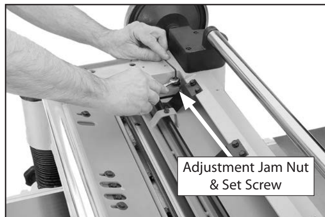
Figure 57. Example of adjusting the pressure bar height.
