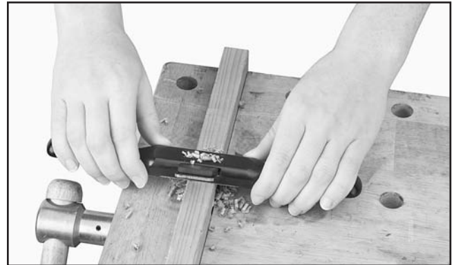
Figure 5. Example of pulling the spokeshave.
