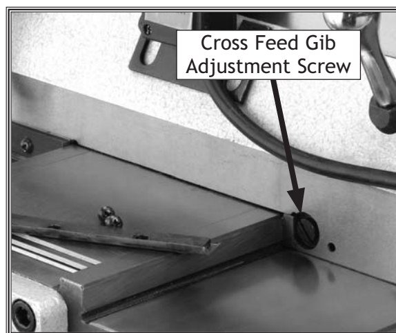
Figure 52. Location of cross feed gib adjustment screw.
