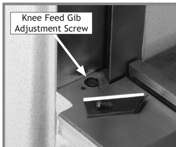
Figure 53. M1003/M1004 knee feed gib adjustment screw.
