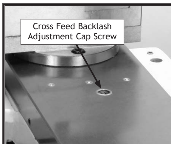
Figure 68. Cross feed backlash adjustment socket head cap screw.
