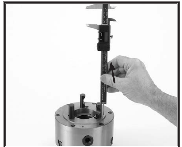
Figure 18. Measuring height of cam-lock studs.
