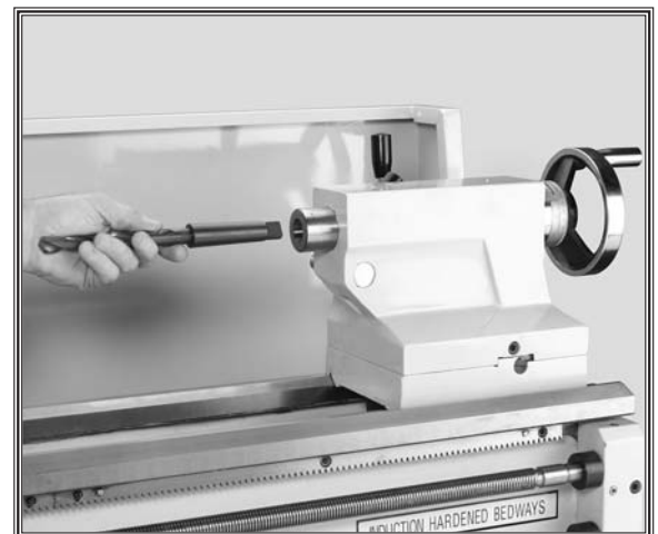
Figure 35. Tapered shank drill fitting into quill taper.
