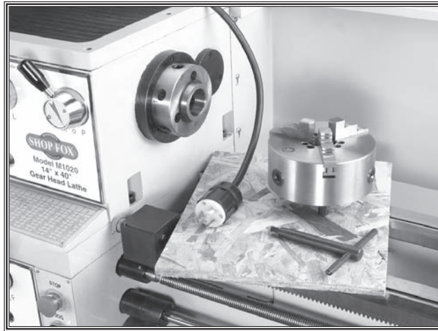
Figure 2. Protecting the bed ways and working safely with electricity.
