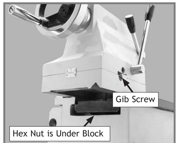
Figure 72. Tailstock nut and gib adjustment.
