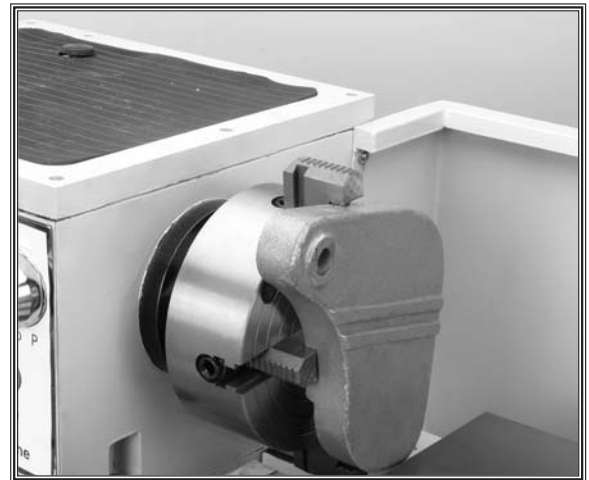
Figure 30. Properly held workpiece for offset machining at low RPM.
