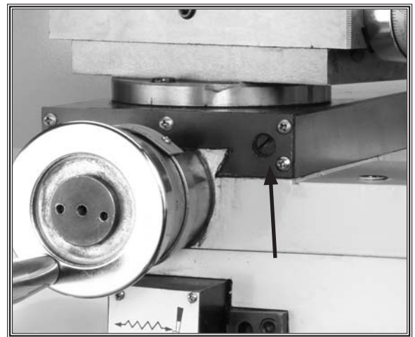
Figure 71. Front cross feed gib screw.
