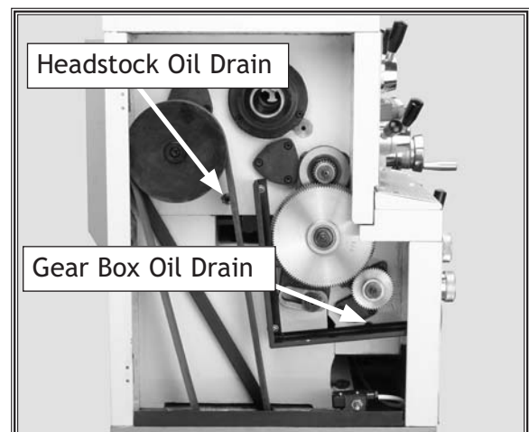
Figure 64. Headstock and gear box drain locations.
