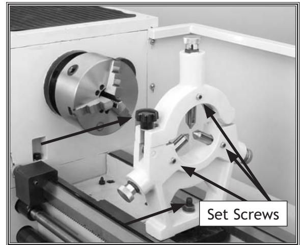
Figure 44. Steady rest adjustments.
