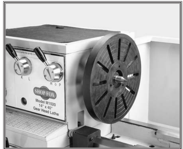
Figure 43. Typical faceplate and dead center setup.
