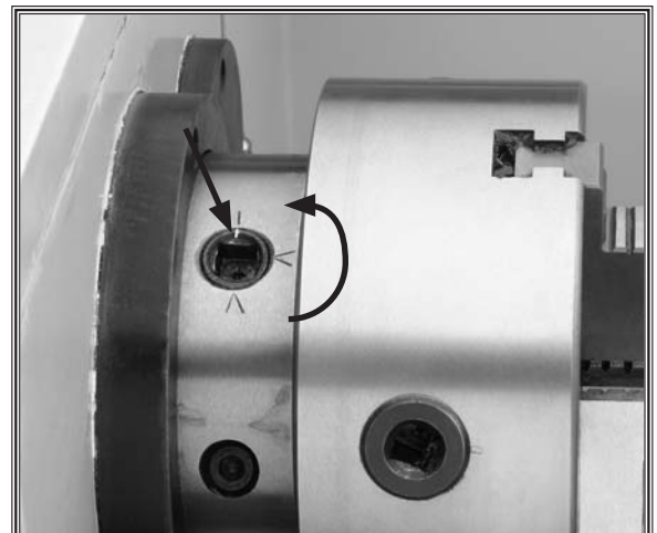
Figure 16. Loosening the cam-locks.
