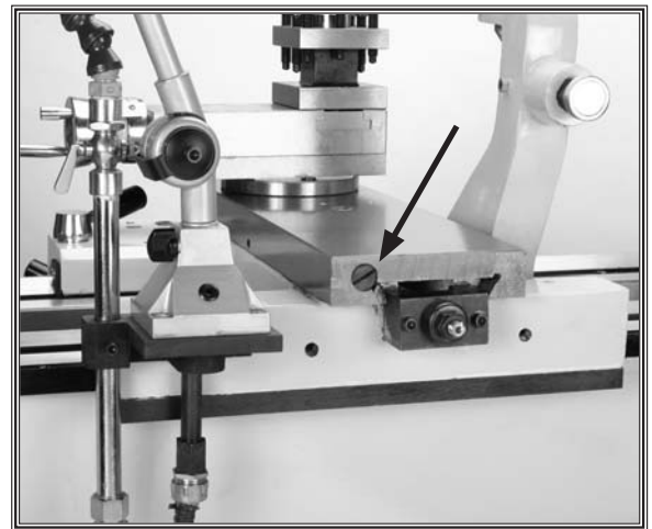
Figure 70. Rear cross feed gib screw.
