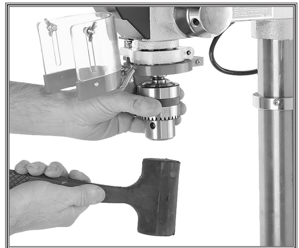
Figure 14. Seating arbor and chuck into spindle.
