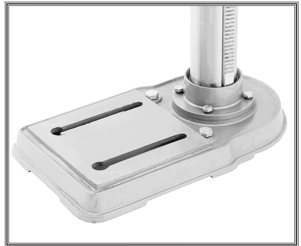
Figure 3. Column secured to base.
