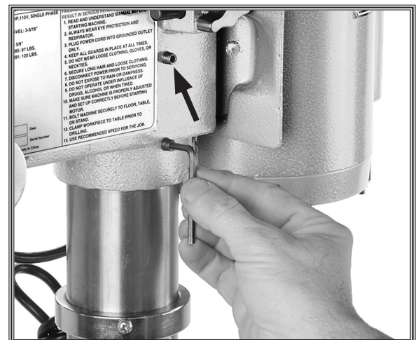
Figure 10. Securing headstock to column.
