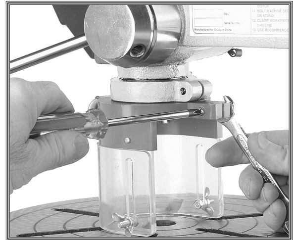
Figure 11. Installing chuck guard.
