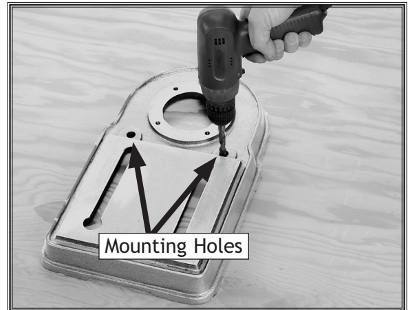
Figure 17. Using holes as a drilling guide.
