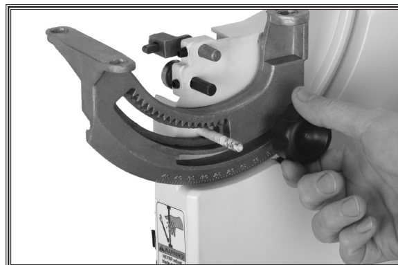
Figure 13. Installing table tilt lock knob.
