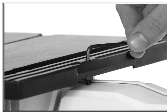
Figure 20. Adjusting positive stop.
