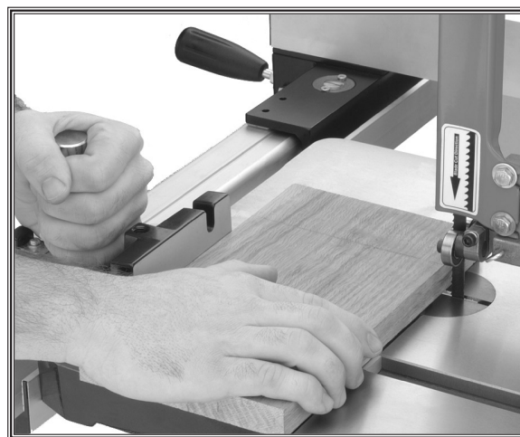
Figure 44. Example of crosscutting operation with miter gauge.
