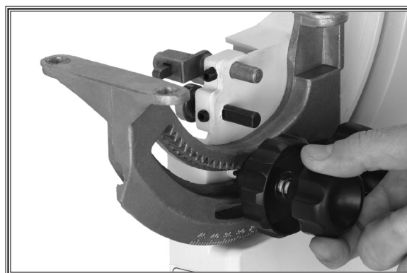
Figure 15. Installing tension knob.
