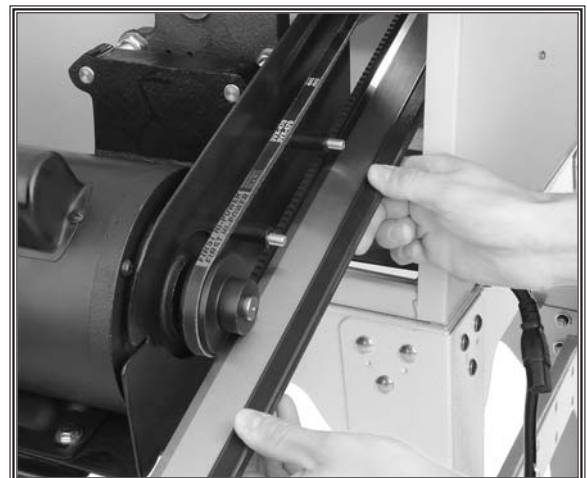
Figure 19. Checking pulley alignment with a straightedge.
