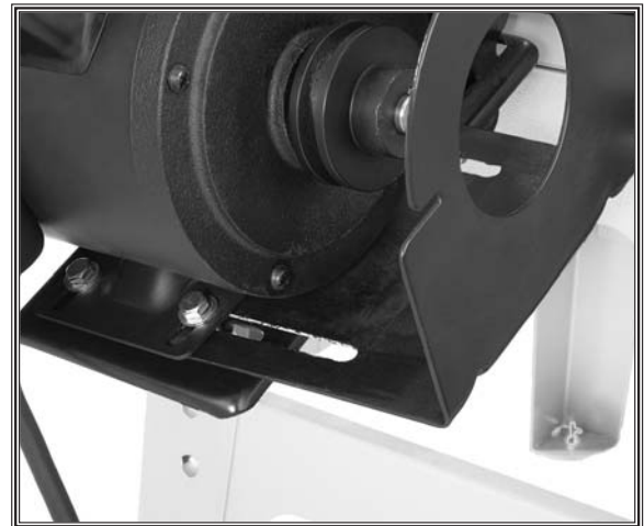
Figure 18. Inserting the pulley guard plate.
