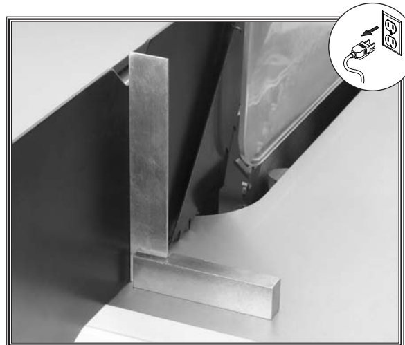
Figure 37. Aligning the splitter with a machinist's square.
