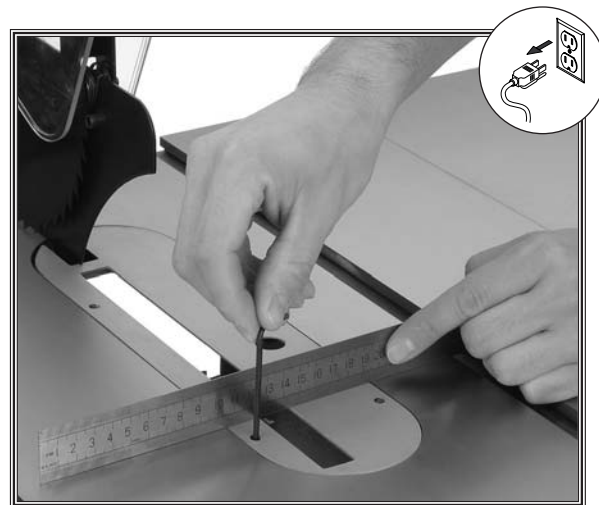
Figure 33. Adjusting table insert height.
