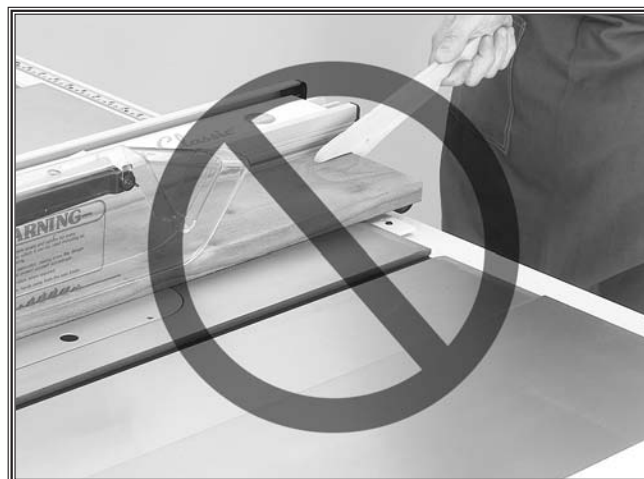
Figure 7. NEVER stand directly behind blade when making a cut.
