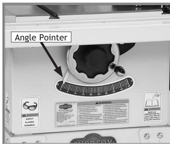
Figure 66. The angle pointer.
