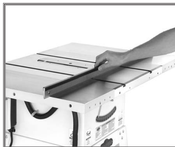
Figure 21. Checking both wings after assembly.
