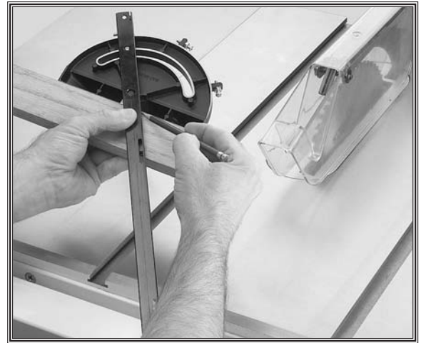
Figure 54. Marking miter line.
