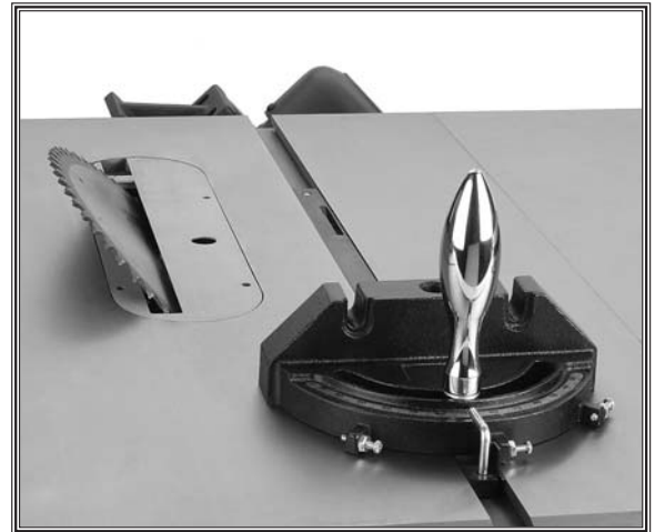
Figure 55. Blade tilted to 45° (guard removed for clarity).
