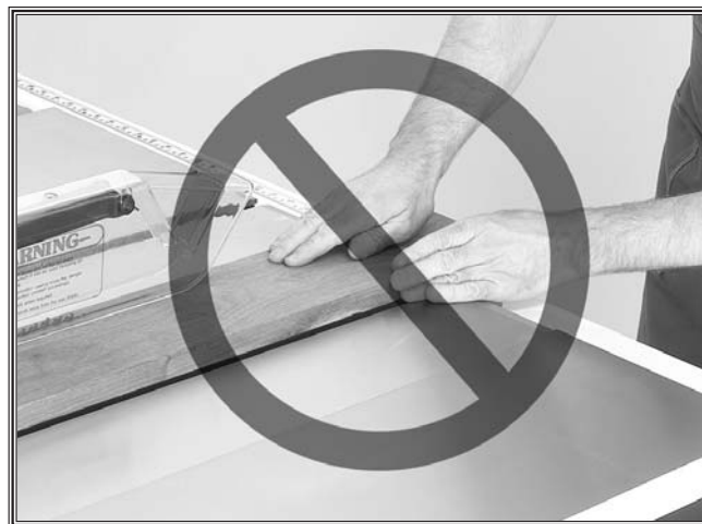
Figure 3. NEVER freehand cut on a table saw.
