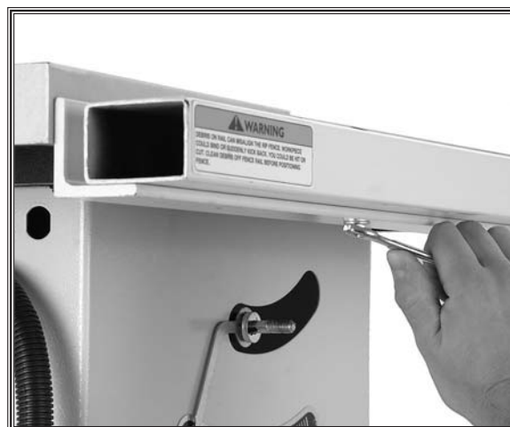
Figure 25. Front rail and fence tube.
