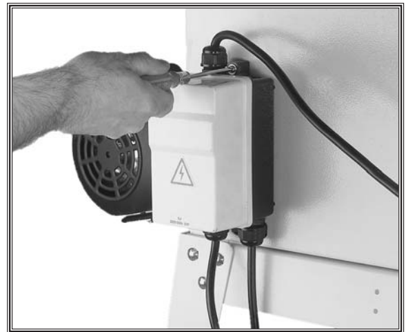
Figure 29. Installing magnetic switch.
