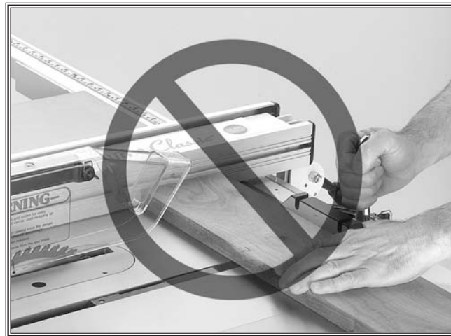
Figure 5. NEVER crosscut using the miter gauge with the fence.
