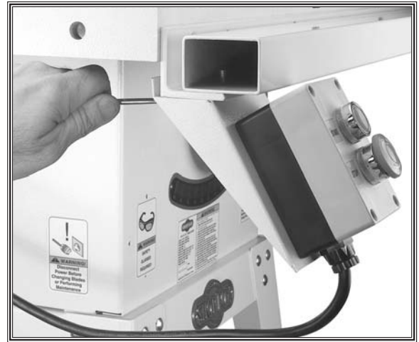
Figure 28. Installing ON/OFF switch.
