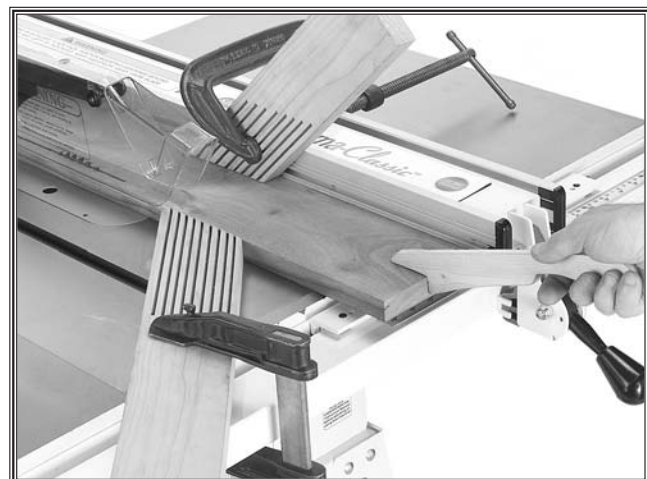
Figure 6. USE featherboards when possible to protect against kickback.
