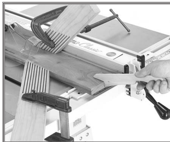
Figure 53. Use a push stick when ripping narrow pieces.
