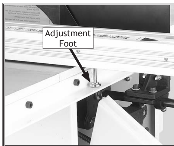
Figure 42. Fence height adjustment.
