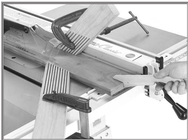
Figure 2. ALWAYS support your workpiece during a cut.
