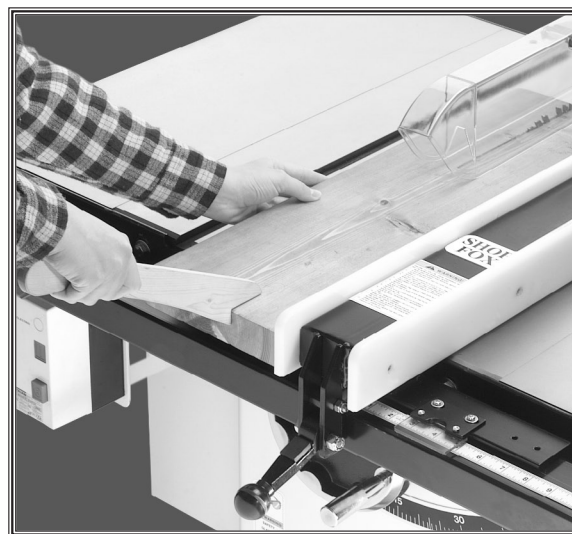
Figure 44. Typical ripping operation.
