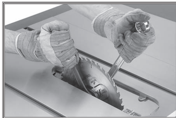
Figure 2. Loosening arbor nut.
