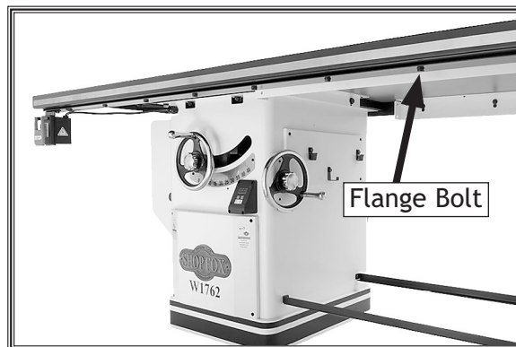
Figure 23. Fence tube mounted to front fence rail.
