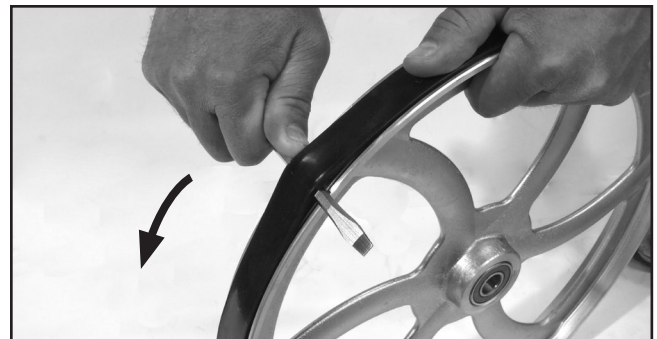
Figure 3. Sliding screwdriver to adjust the placement of the tire.
