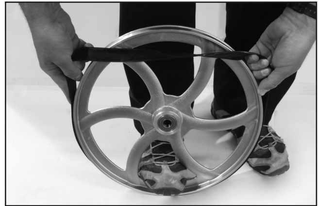
Figure 2. Installing the tire on the wheel.
