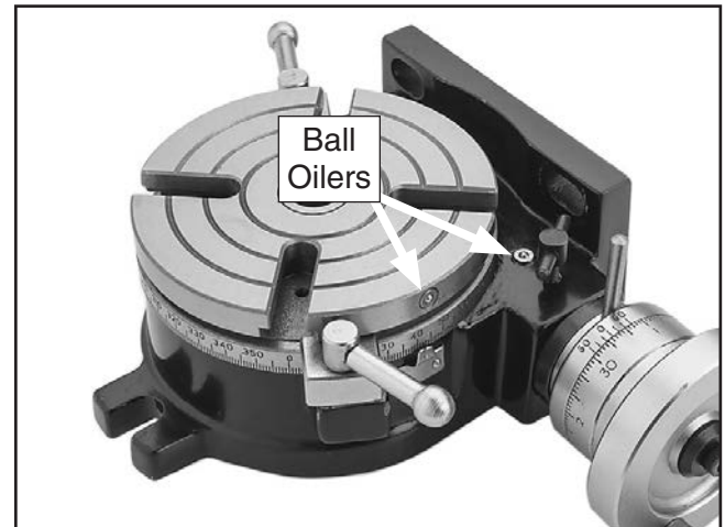
Figure 41. Location of ball oilers.
