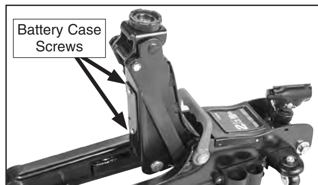
Figure 7. Battery case location.
