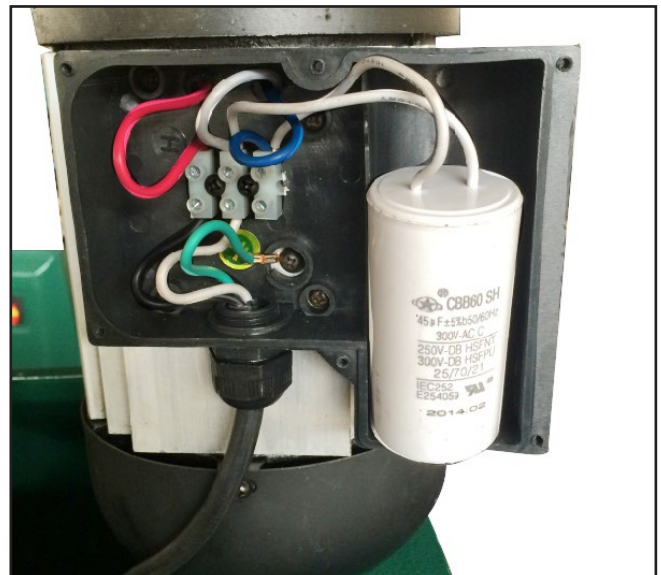
Figure 29. T26418 motor connections.
