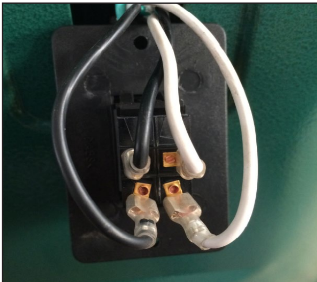
Figure 28. T26418 switch connection.
