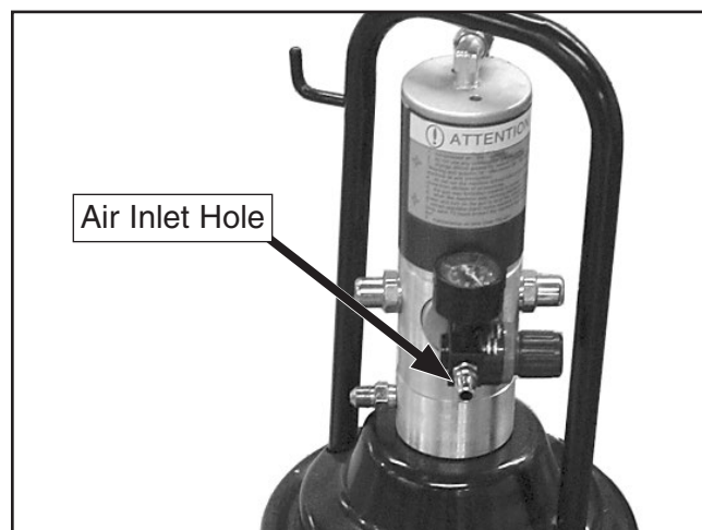
Figure 7. Location of air inlet hole where air-pump lubricant is added.
