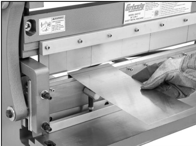
**Figure 31.** Positioning workpiece for bend.
