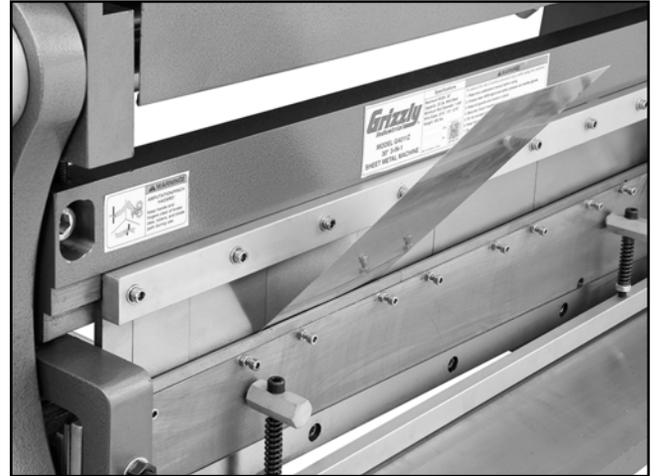
**Figure 32.** Bending workpiece.
