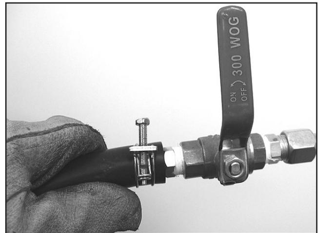
**Figure 11.** Blast nozzle valve, closed.
