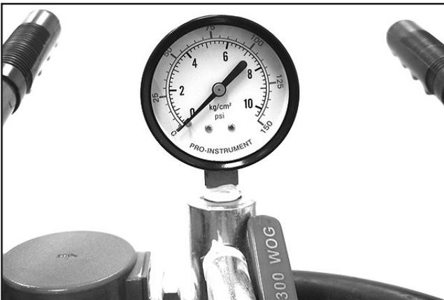
**Figure 10.** Tank air pressure at zero PSI.
