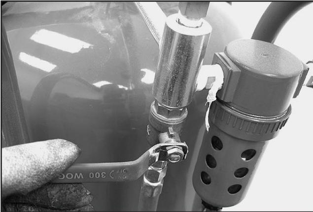
**Figure 9.** Blast hose air supply valve, closed.
