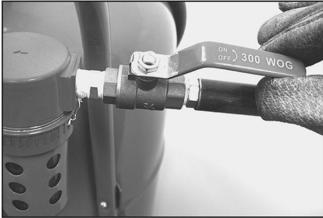
**Figure 12.** Tank air supply valve, opened.
