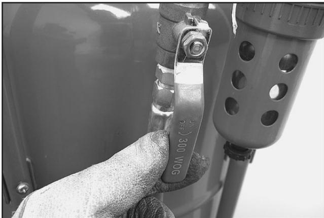
**Figure 13.** Blast nozzle air supply valve, opened.
