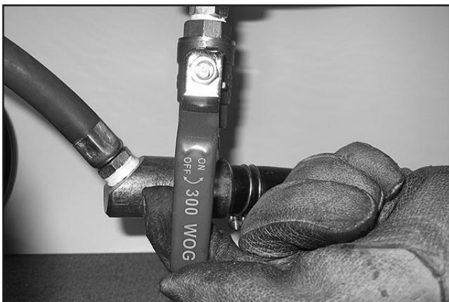
**Figure 14.** Sand metering valve in the full-open position.
