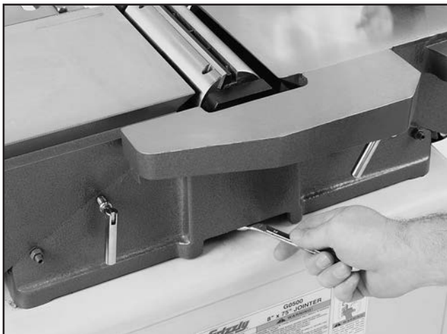
Figure 3. Example of removing nut and lock washer on bearing block stud.
