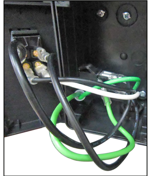
Figure 65. ON/OFF switch and 110V outlet wiring.
