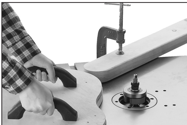
Figure 56. Example of using a jig with a starting block.
