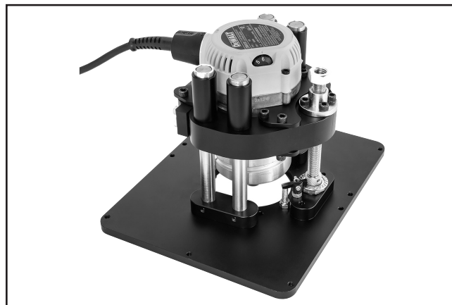
Figure 37. Example of router installed in clamping plates.
