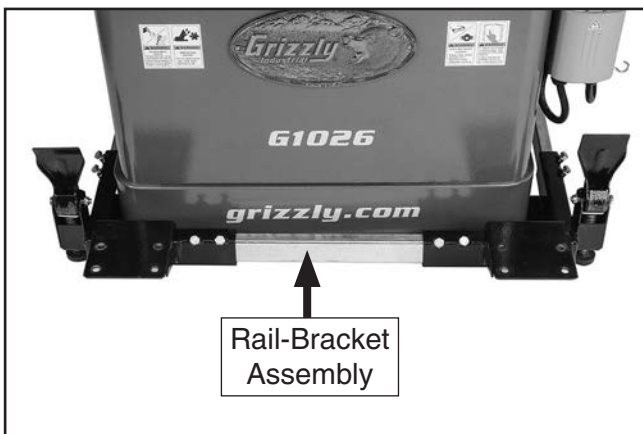
Figure 17. Rail-bracket assembly placed under front of machine.
