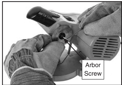
Figure 6. Holding blade in place to remove arbor screw.
