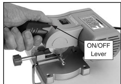
Figure 9. ON/OFF lever during cut.
