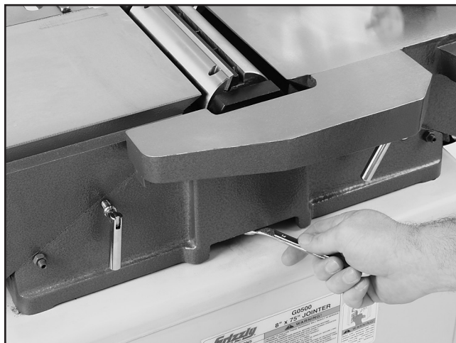
Figure 3. Example of removing hex nut and lock/flat washer on bearing block stud.
