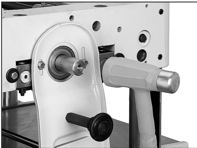
Figure 8. Unseating cutterhead from headstock.
