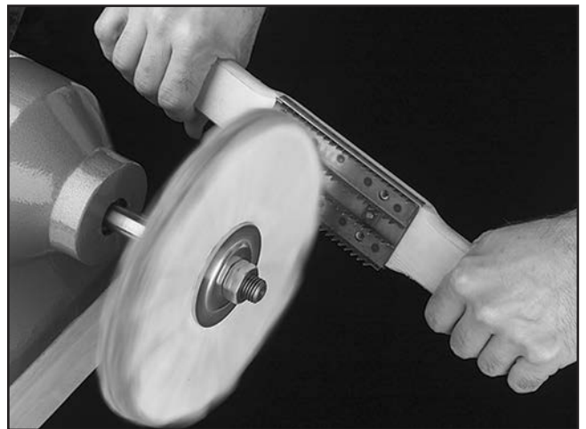
Figure 20. Removing compound from buffing wheel with buffing wheel rake.
