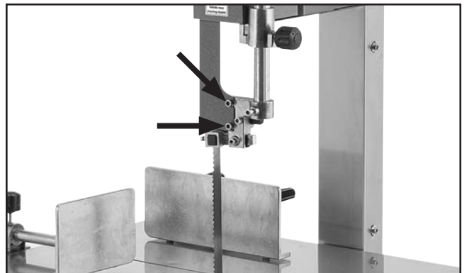
Figure 42. Cap screws securing blade guard.
