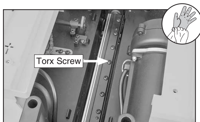
Figure 8. T-30 Torx screws on knife clamp.
