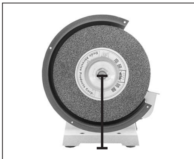
Figure 3. Example of distance to measure (wheel guard removed for clarity).
