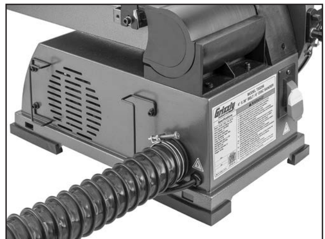
Figure 14. Dust hose attached to dust port.
