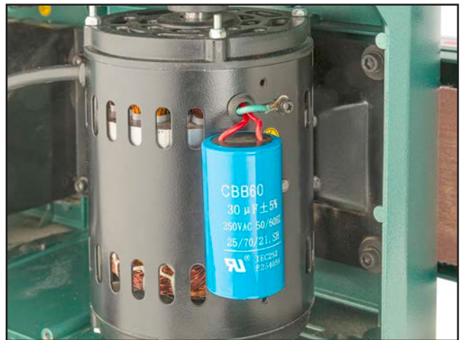
Figure 70. Run capacitor wiring.
