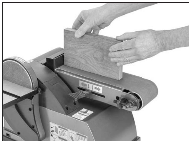
Figure 38. Properly sanding workpiece edge.
