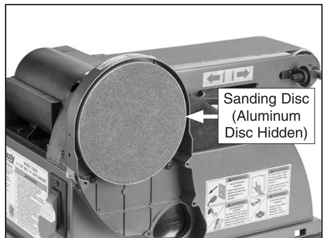
Figure 25. Sanding disc stuck to aluminum disc.
