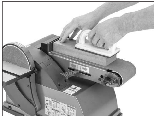
Figure 37. Properly sanding workpiece face.
