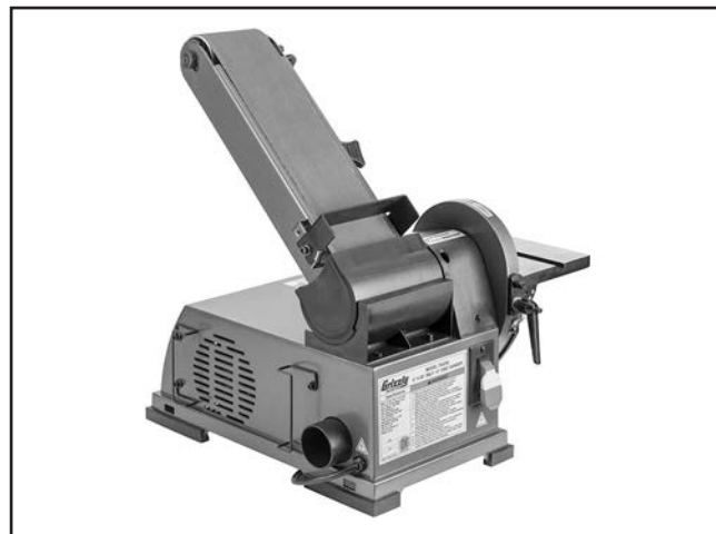
Figure 21. Platen positioned at 45°.
