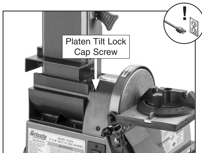
Figure 22. Location of platen tilt lock cap screw.
