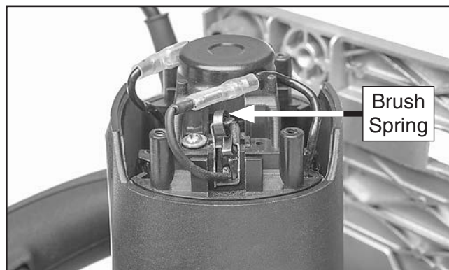
Figure 33. Motor brushes installed.
