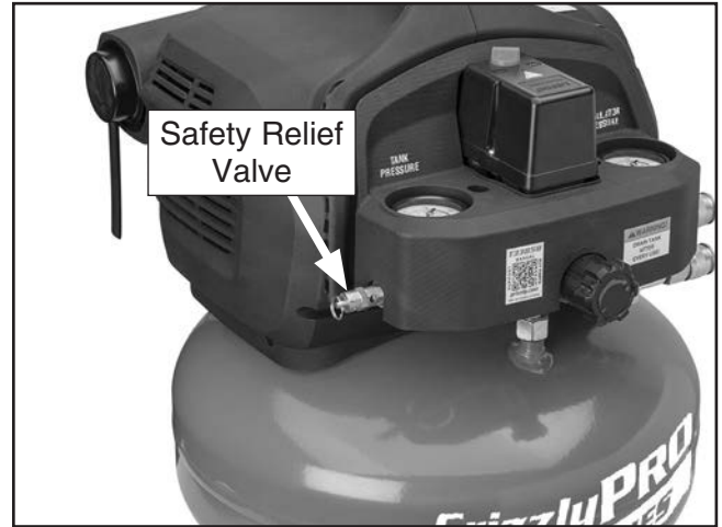
Figure 12. Location of safety relief valve.
