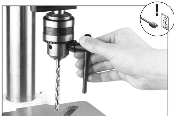
Figure 35. Example of tightening chuck with chuck key.
