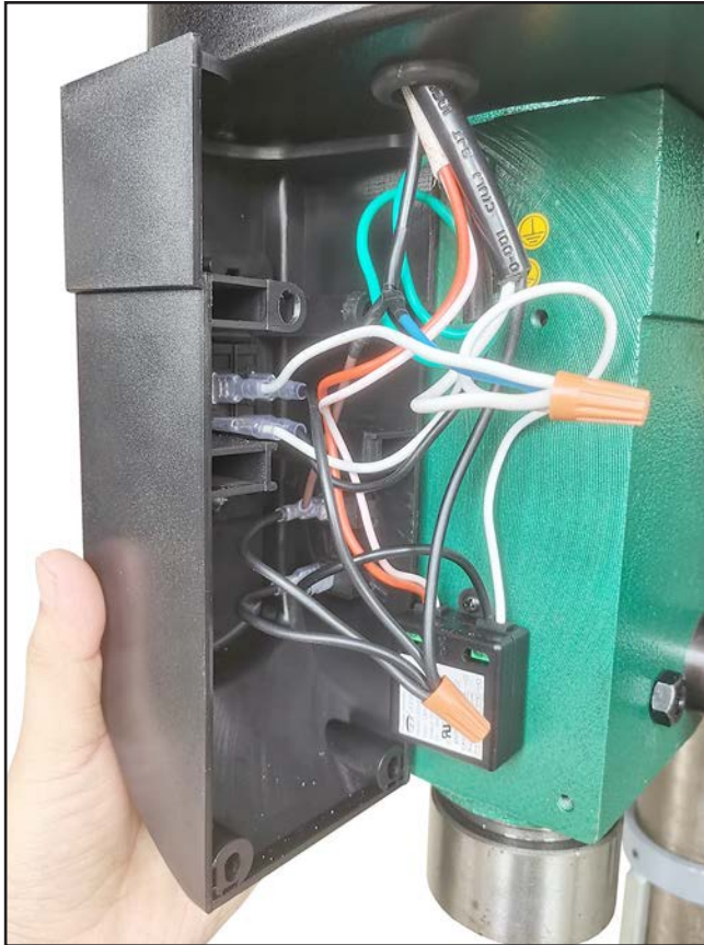
Figure 67. Switch box wiring.
