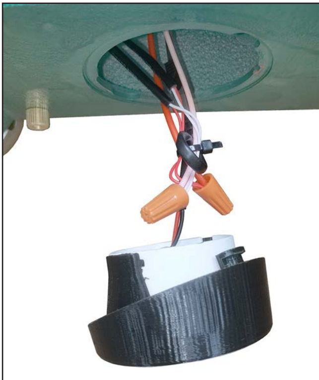
Figure 68. LED & laser module wiring.
