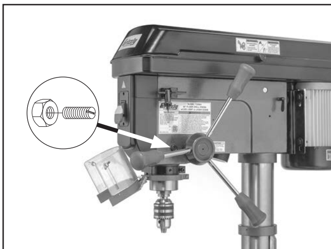
Figure 66. Location of quill shaft lock screw and jam nut.
