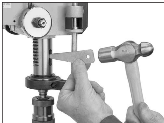
Figure 30. Example of using drift key to remove arbor from spindle.
