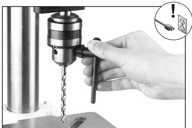
Figure 35. Example of tightening chuck with chuck key.
