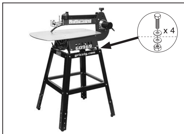
Figure 8. G0969 Scroll Saw mounted on stand.
