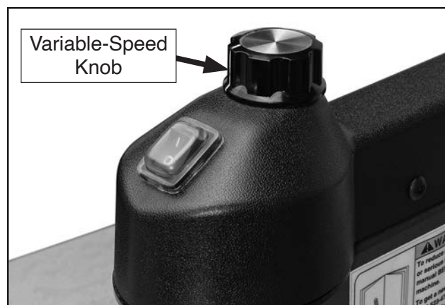
Figure 21. Location of variable-speed knob.
