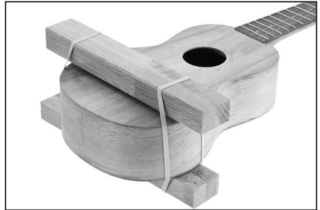
Figure 18. Bridge secured with wood blocks.
